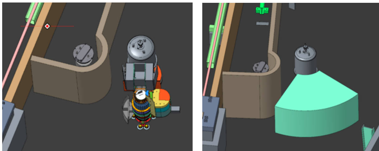
Figure 10. Schematic view of MANTA with single analyzer (left) and multiplex analyzer (right).
