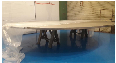
Bottom plate welding completed
