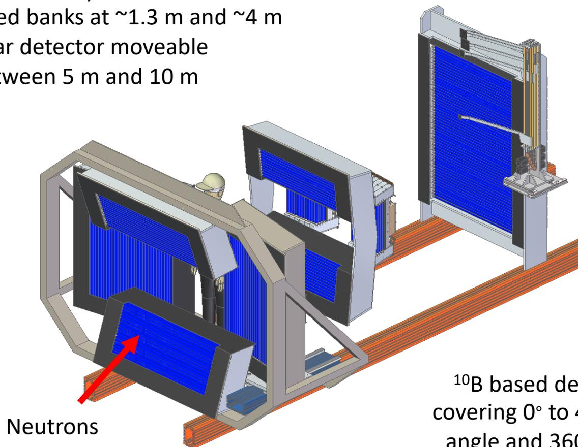
$^{10}\text{B}$  based detector system covering  $0^\circ$  to  $45^\circ$  in scattering angle and  $360^\circ$  in azimuthal angle ( $180^\circ$  Day 1).
