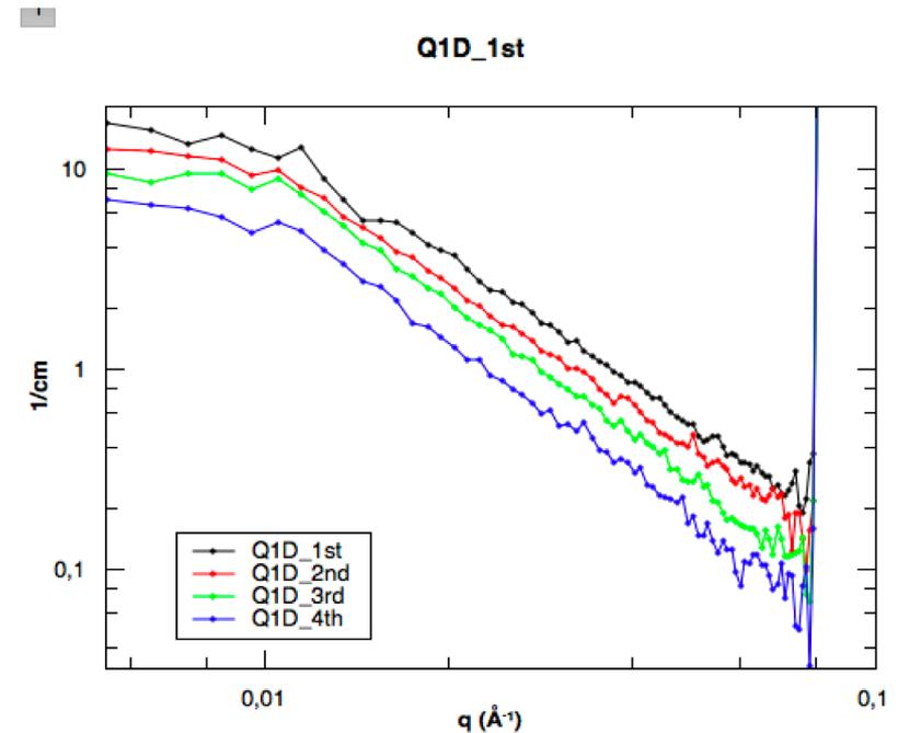
Convert units (to wavelength)  $\rightarrow$  **Normalise to monitor**  $\rightarrow$  Extract spectrum (e.g. the back detector spectra)  $\rightarrow$  rebin  $\rightarrow$  Q1D with the appropriate binning (e.g. 0,0.001,0.2)
