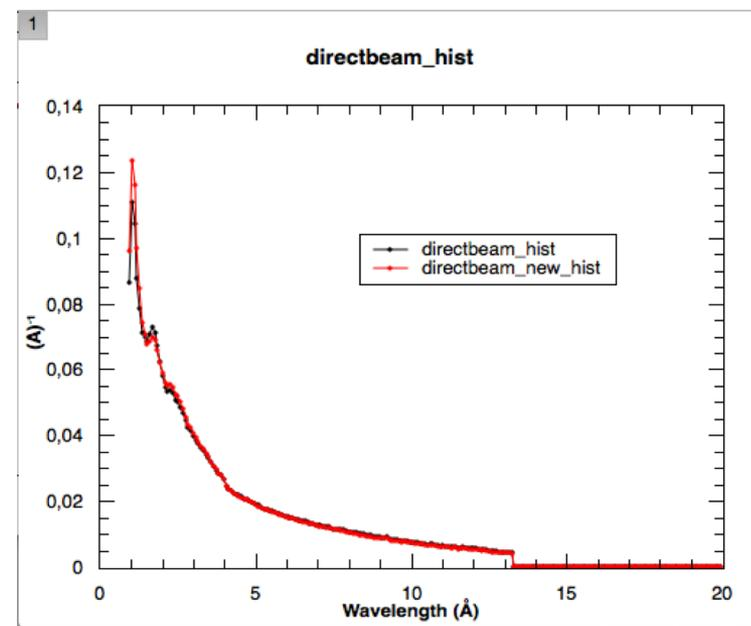
The “direct beam” is the relative efficiency of the main detector compared to the monitor
