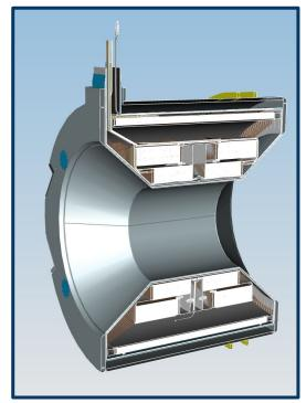
Strong 5T solenoid already incorporated into the detector system of CLAS12.
