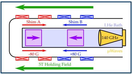
But the sharp change in magnetic field increases the required currents and demands a more precise coil design.
