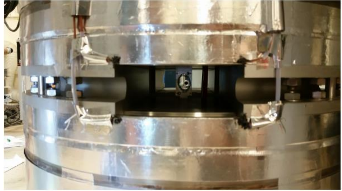
Type-T Thermocouple sensors are installed upstream/downstream of the magnet
