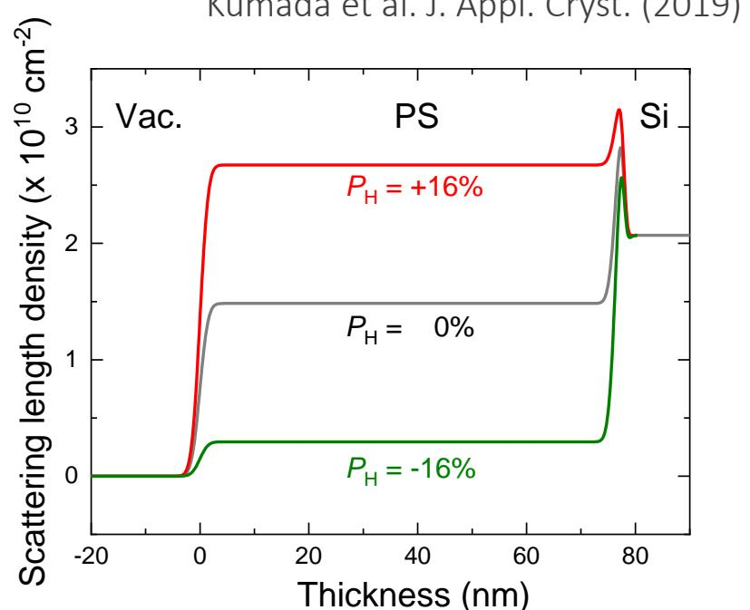
Homogeneously polarized including surface and interface
