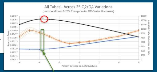
Maximization of the rate necessitates increasing the flux of electrons passing through the dipole box to its maximum. In this design, maximizing the rate is quivalent to maximizing the e- flow through the dipole which means bringing the envelope edge close to the dipole outer wall.
