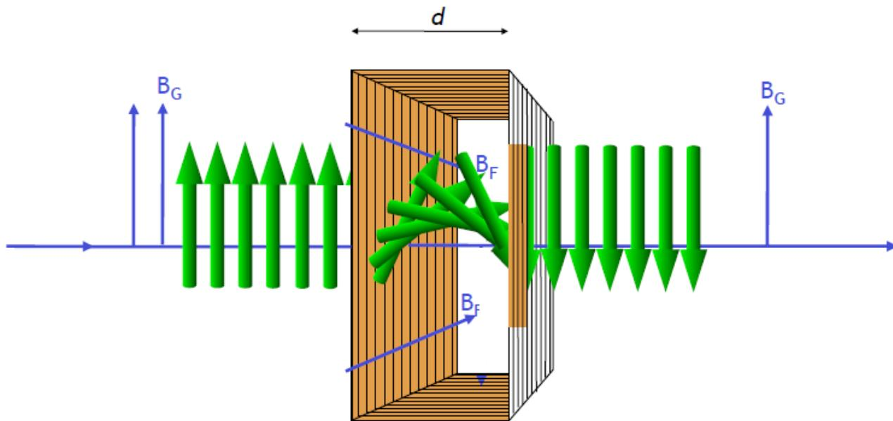
A flip of  $\phi$  radians with respect to the guide field can be achieved if the resultant field within the coil,  $B_F$ , is perpendicular to  $B_G$  and
