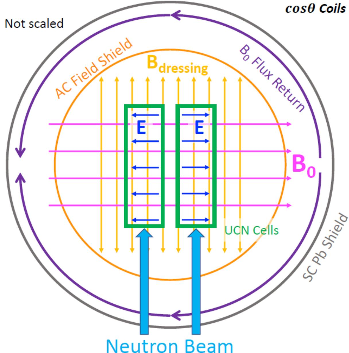
**B<sub>0</sub> Coil:** (Superconducting Cu-clad NbTi wire)
