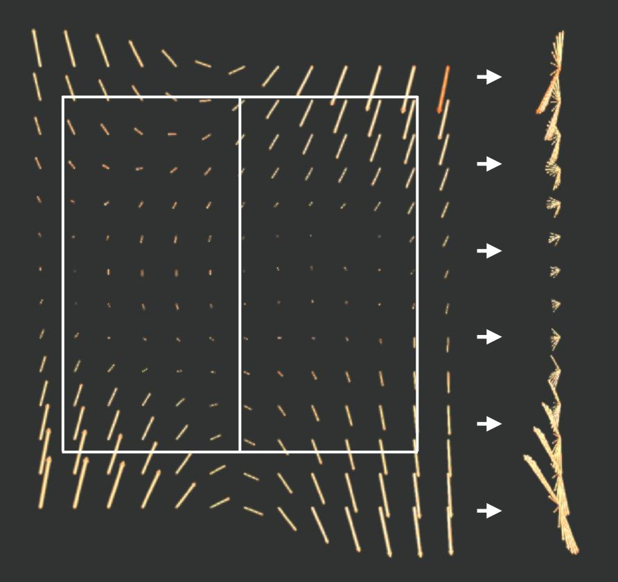
Highly contained B-Field with low leakage fields (<mG at 1in)
