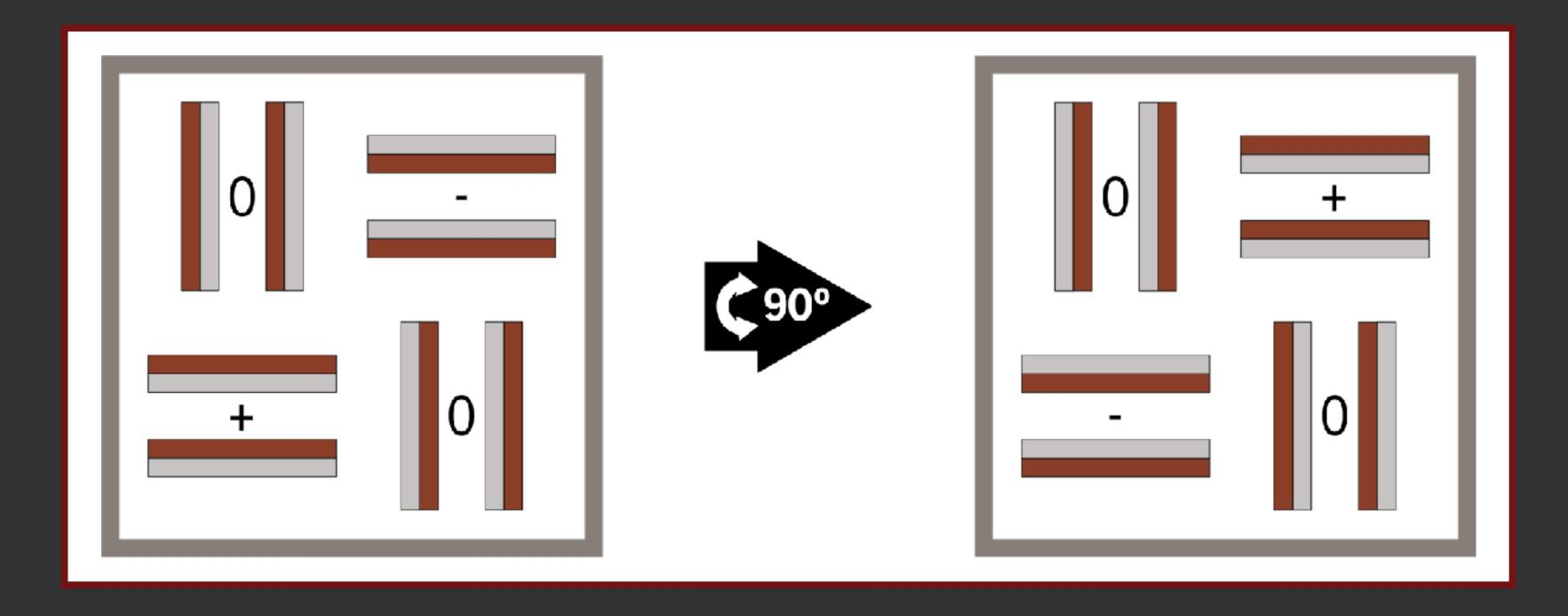
Target rotation needed for constraint of systematics — Geneva gear incorporated into vacuum end cap to implement discrete rotations
