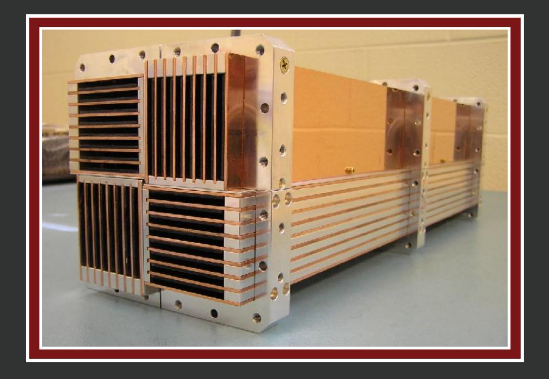
Copper and float glass plates spaced with asymmetric density in each slot
