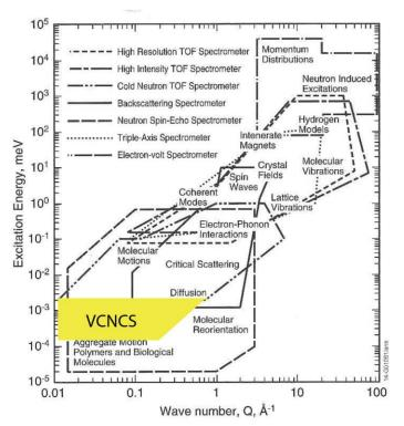
Yellow shows the range of Q-E space accessible by reducing the incident energy available on the CNCS instrument by an order of magnitude, perhaps enabled by a VCN source. This region might enable studies of soft matter presently in the domain of spin echo.
