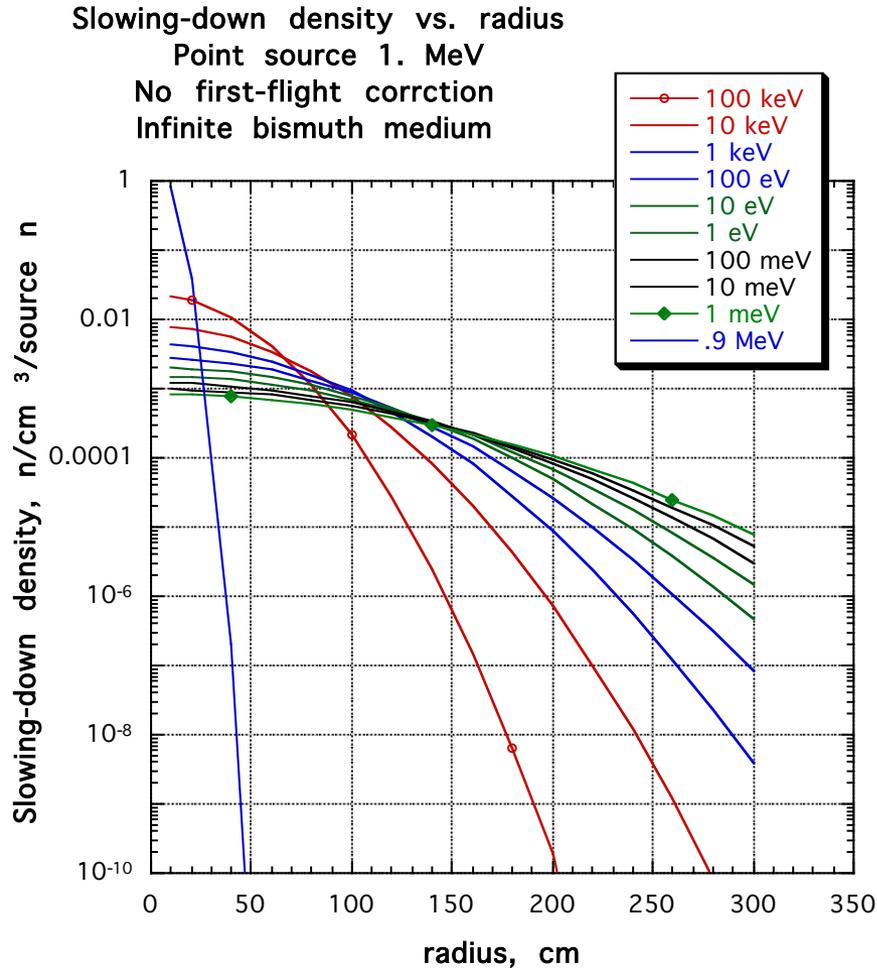
The figure shows the slowing-down density,  $q(r,E)$ , of neutrons from a point source in an infinite medium of bismuth, calculated from classical theory.
