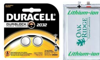
Fig. 5.18. Shown at left is a coin cell where the amount of active cathode material is 0.01 g. At right is a pouch cell specially manufactured to understand the behavior of the cathode as a function of cycling using POWGEN. The active cathode material here is 1 g.
