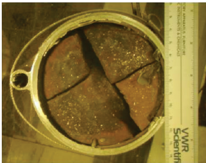
Fig. 8.1. Photograph of the upper portion of the opened MK 0 Lujan target following service, as viewed from the impinging beam [1].
