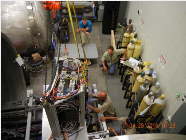
Figure 11: Securing the detector to the carriage
