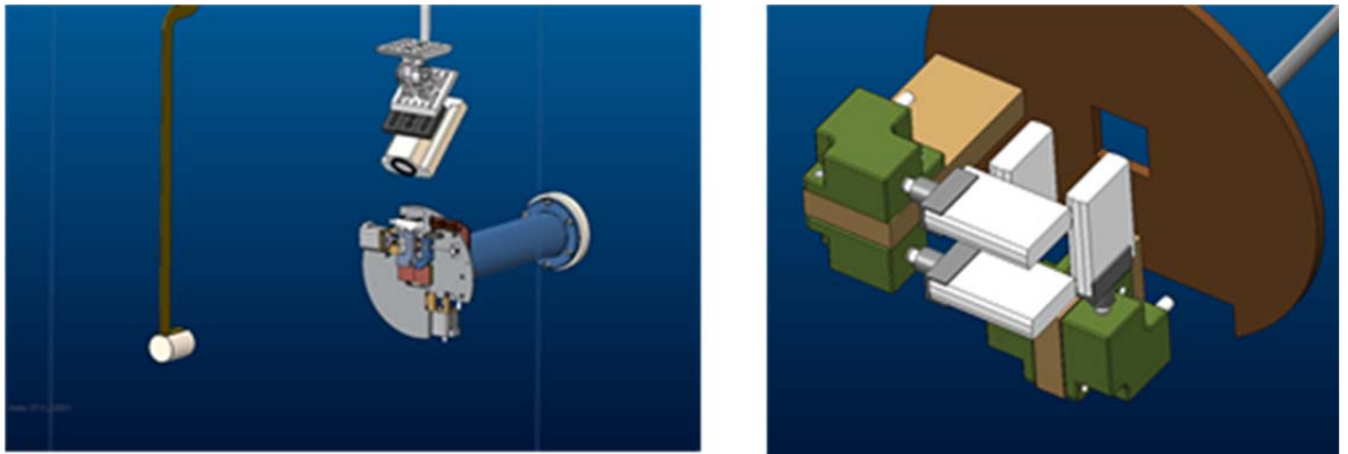
Figure 1: Concept drawing of beam defining slit option for NOMAD
