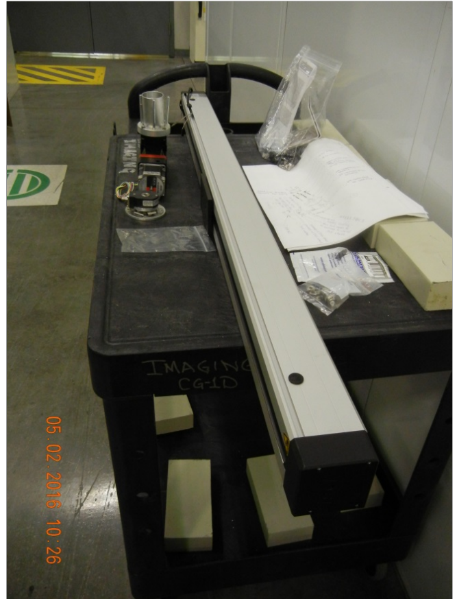
Figure 16: Calibration arm, gear box and encoder
