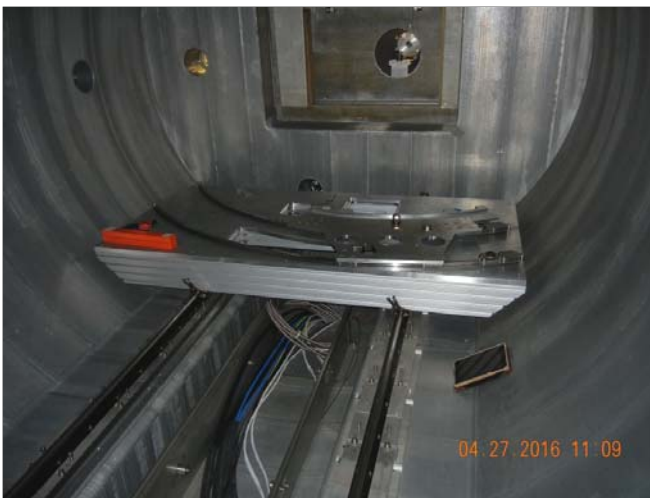
Figure 9: Alignment of detector plate in carriage
