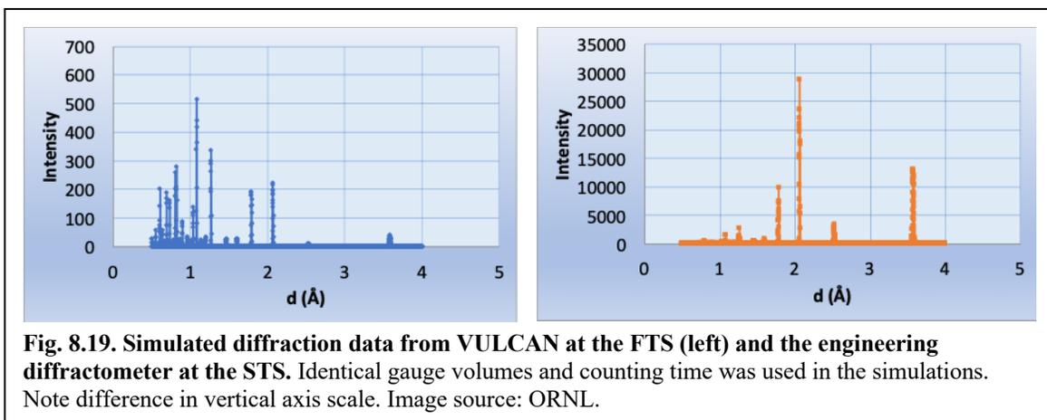
high-wavelength resolution of thermal neutrons available on the FTS to study high-symmetry crystal structures. Table 8.8 lists key parameters of the proposed instrument.
