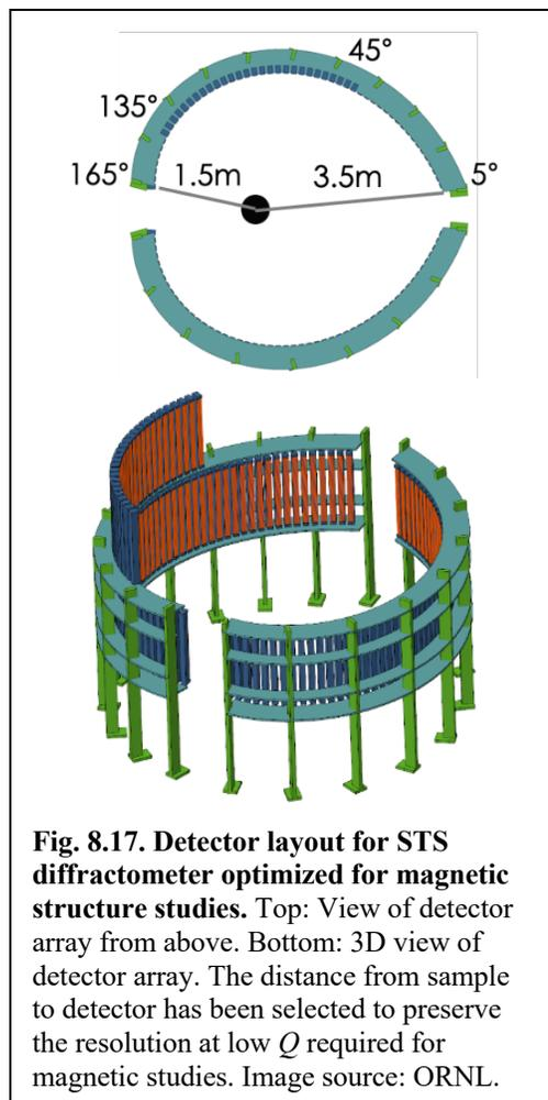
**Fig. 8.17. Detector layout for STS diffractometer optimized for magnetic structure studies.** Top: View of detector array from above. Bottom: 3D view of detector array. The distance from sample to detector has been selected to preserve the resolution at low  $Q$  required for magnetic studies. Image source: ORNL.
