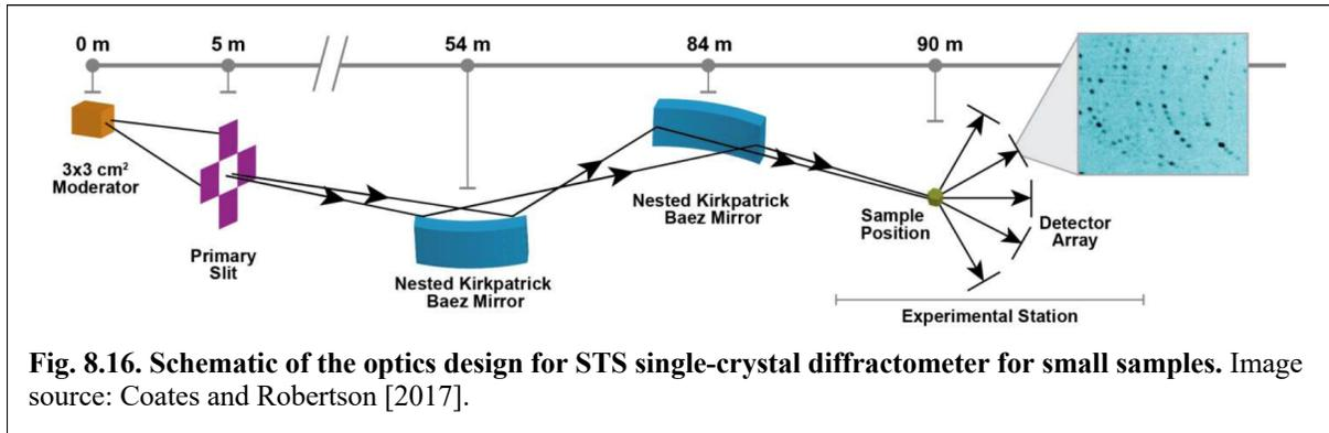
**Fig. 8.16. Schematic of the optics design for STS single-crystal diffractometer for small samples.** Image source: Coates and Robertson [2017].
