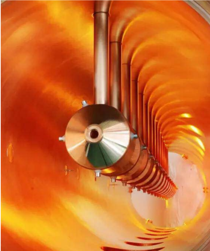
All drift tubes have been installed
