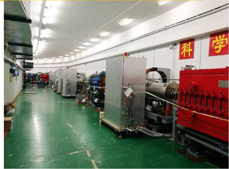
RCS RF-cavity Installation
