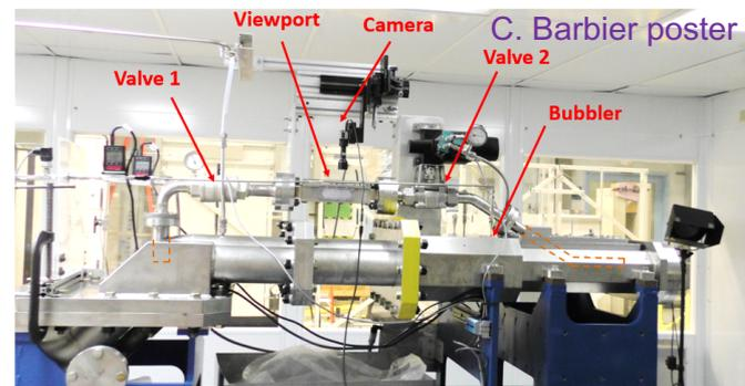
TTF target with its sampling setup to measure bubble size distribution
