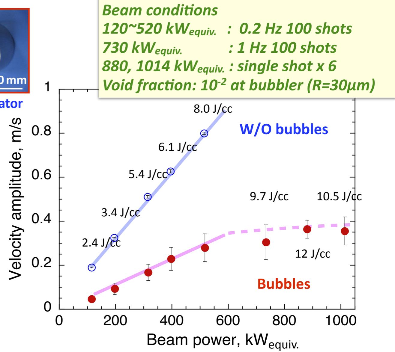
*LDV peak amplitude obtained from 7th target*
