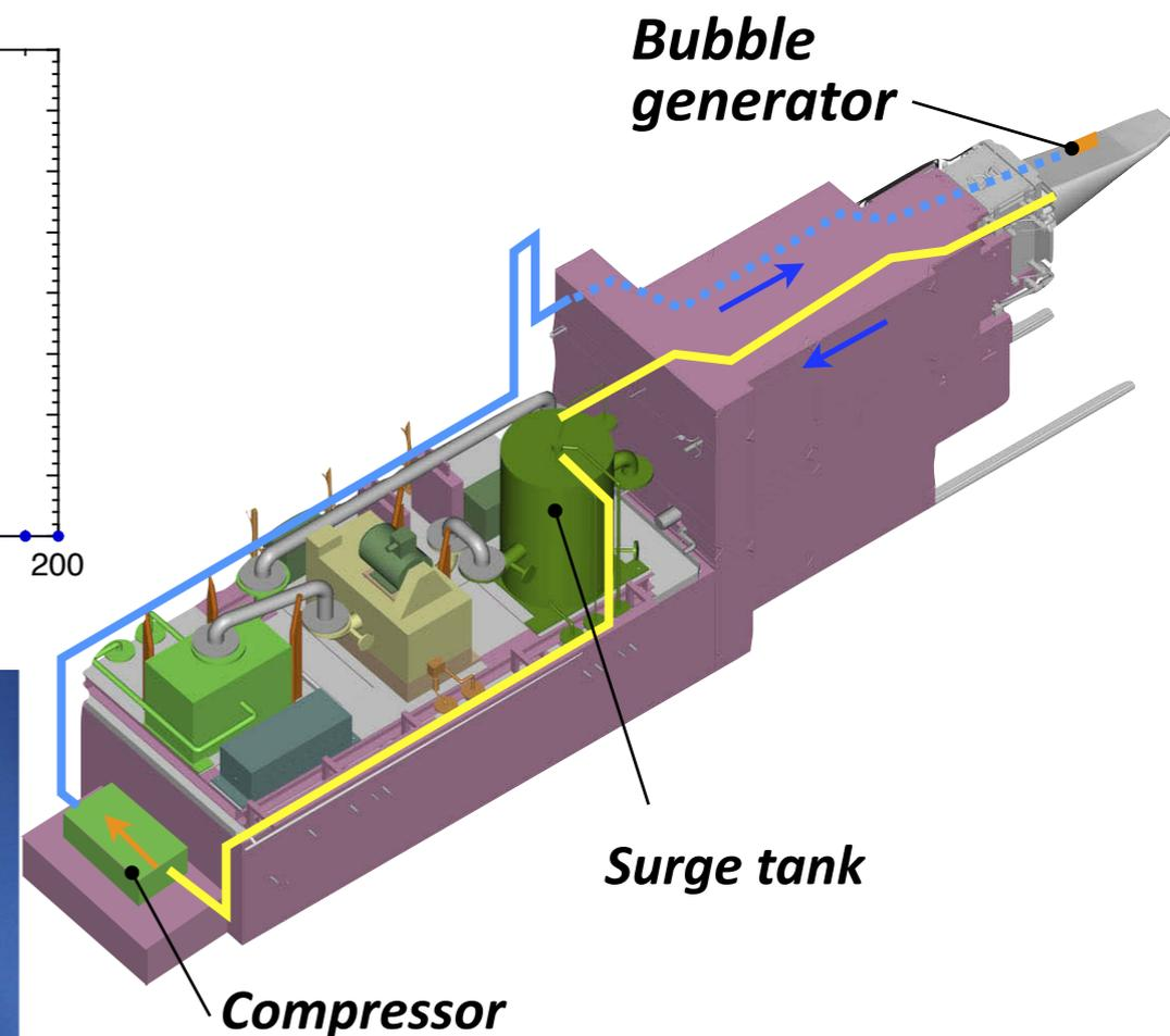
*JSNS mercury circulation system (Closed helium gas loop)*
