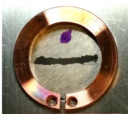
Coin 3 mm thick Flux \sim 1\text{e}10 ions/s/cm 2 Fluence 1\text{e}14 i/cm 2
