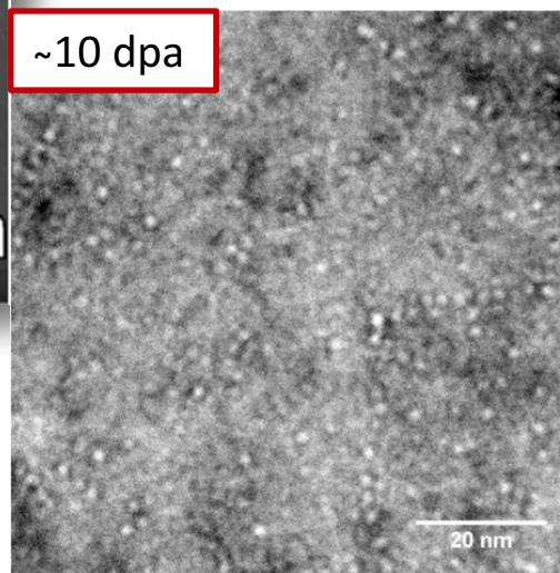
Early stage displacement damage, He-V clusters; almost no experimental data from electron microscopy techniques
