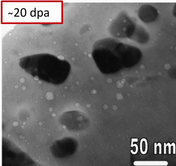
Severe displacement damage, large He bubbles; He bubbles can be well characterized by TEM and STEM/EELS; Lot of experimental data – good level of understanding
