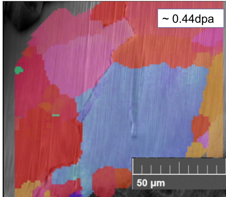
Transition from transgranular fracture to grain boundary/mixed mode fracture
