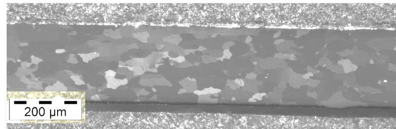
Surface normal-projected inverse pole figure orientation map, with high angle grain boundaries
