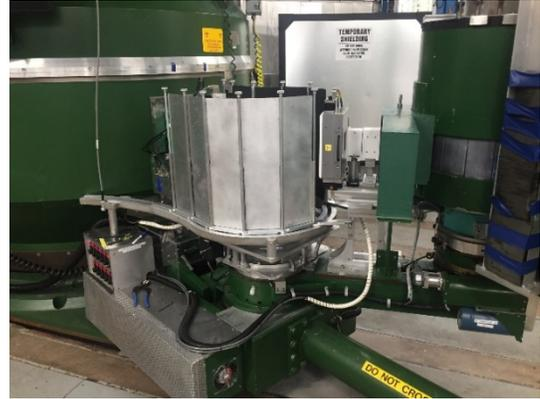
Figure 3.10. Shielding design around the HB-3 sample position.
