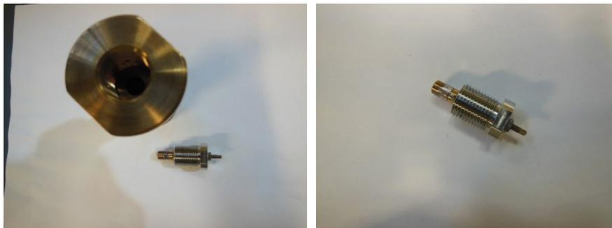
Figure 11.15. Photos of a CuBe gas pressure capable of 3 kbar available on VISION. The gas pressure cells is also H<sub>2</sub>/D<sub>2</sub> compatible
