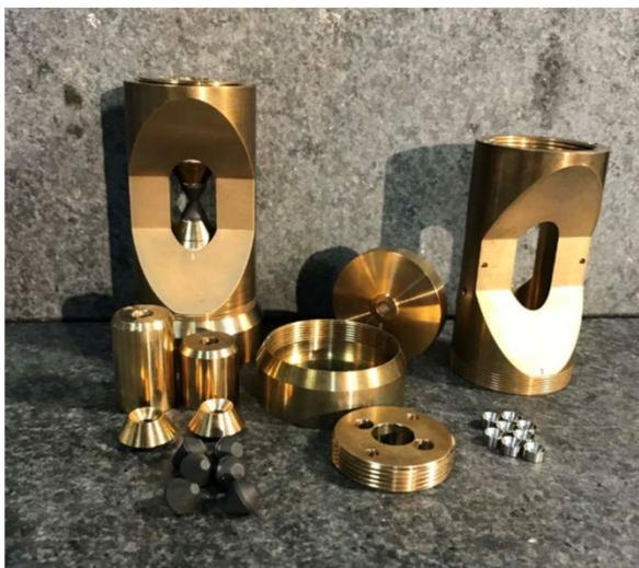
Figure 11.16. CuBe clamped diamond cells with Versimax® anvils.
