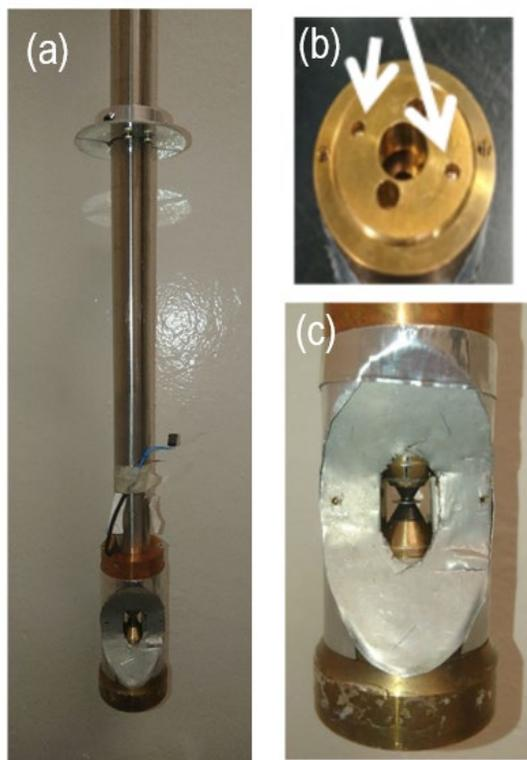
Figure 11.17. Three images of VISION clamped DAC: (a) mounted on the new sturdy stick, via (b) two bolt holes on the DAC cap and (c) a close-up of the DAC with its cadmium shielding.
