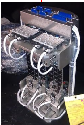
Doubly focusing analyzer assembly provided by Japanese collaborators
