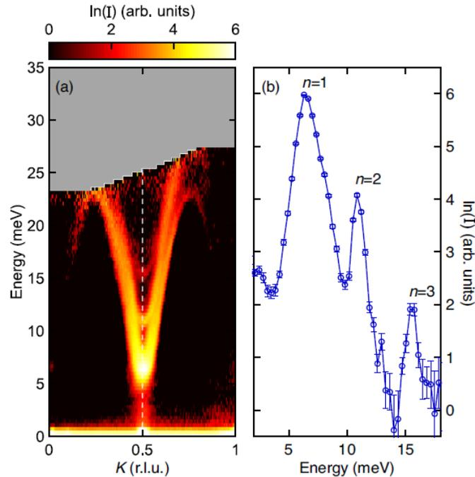
(a) Measured excitation spectrum of  $\alpha$ -NaMnO<sub>2</sub> and (b) cuts through the antiferromagnetic zone center (white dashed line in (a)) demonstrating the observation  $n=1$ ,  $n=2$ , and  $n=3$  magnon modes.
