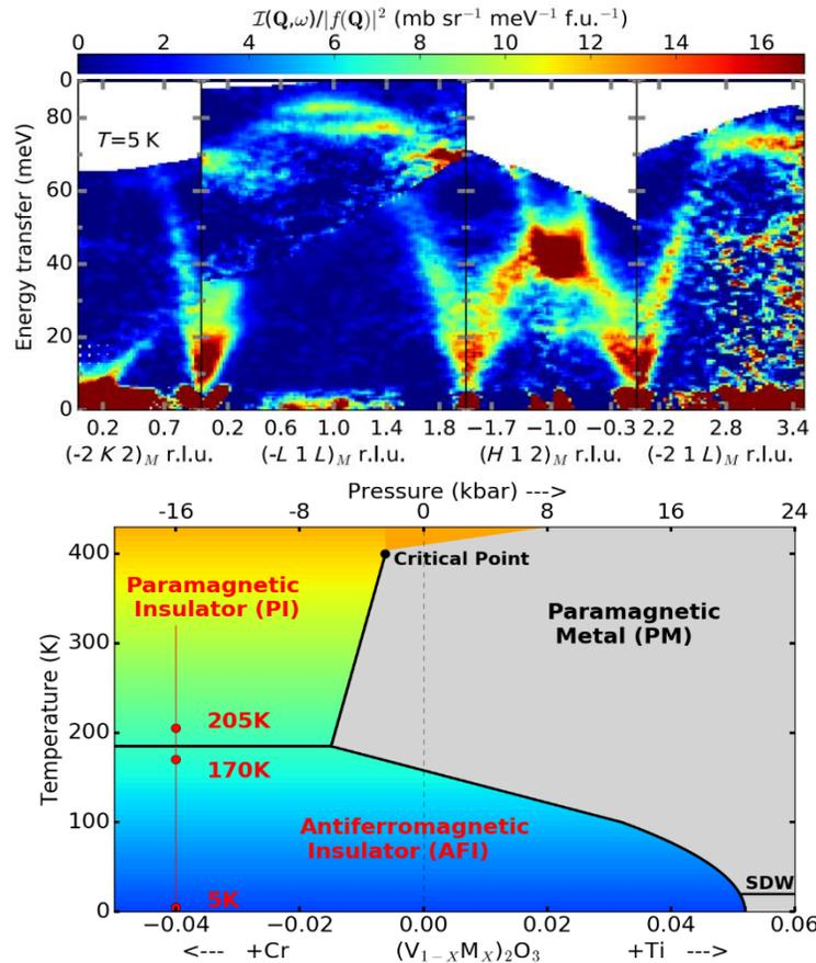
(Top) Neutron scattering from spin waves across four high symmetry directions. (Bottom) Phase diagram of  $V_2O_3$  indicating the paramagnetic-insulating phase originating from frustrated magnetic interactions.
