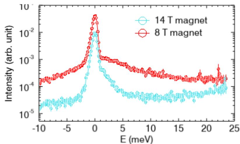
**Empty 14 T magnet has ~5 times less background than the 8 T magnet**
