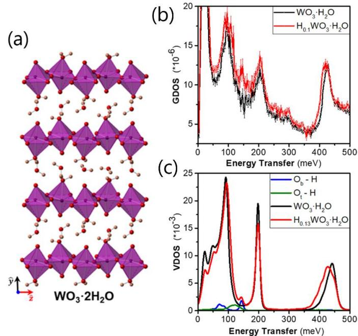
(a) Crystal structure of monoclinic  $\text{WO}_3 \cdot 2\text{H}_2\text{O}$  showing the interlayer water. (b) Generalized vibrational density of states (GDOS) from INS and (c) ab initio molecular dynamics simulations of the vibrational density of states (VDOS) establish the locations of protons in the material.
