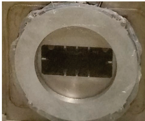
Figure 4.33. FTS halo monitor as mounted in PBW assembly.
