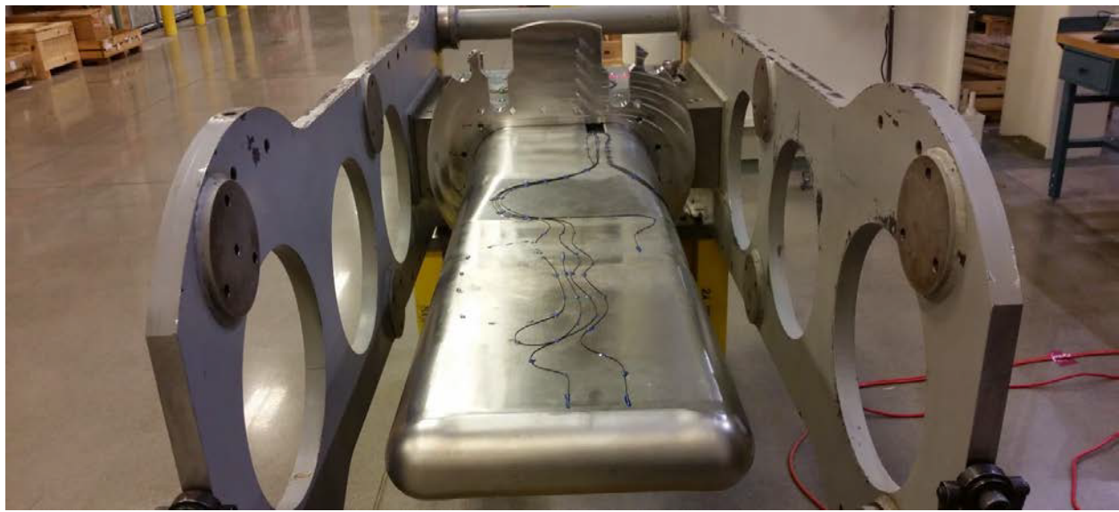
Figure 1. Strain Sensors Mounting to Target Module. Note that the Water Shroud is removed.
