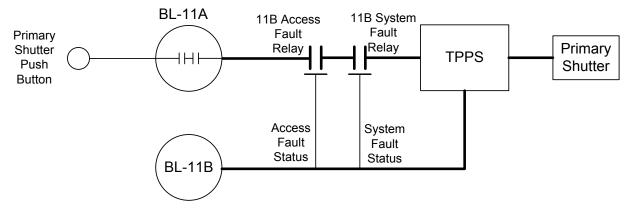
The relays will be physically located in the TPPS-Cab07 control cabinet as shown on modified drawings 109090201-R8U-8700-A117, Rev1 and 109090201-R8U-8700-A105, Rev1. The relays will add the fault statuses from BL-11B to the Primary shutter "Open" request signal that is generated at BL-11A and sent to TPPS.
