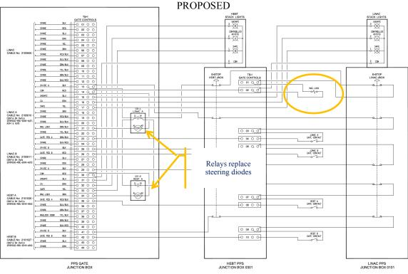
Figure 5 Modified gate maglock control using relays for isolation
