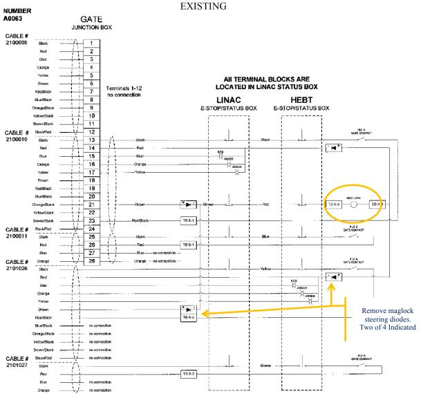
Figure 4 Existing gate maglock control using steering diodes
