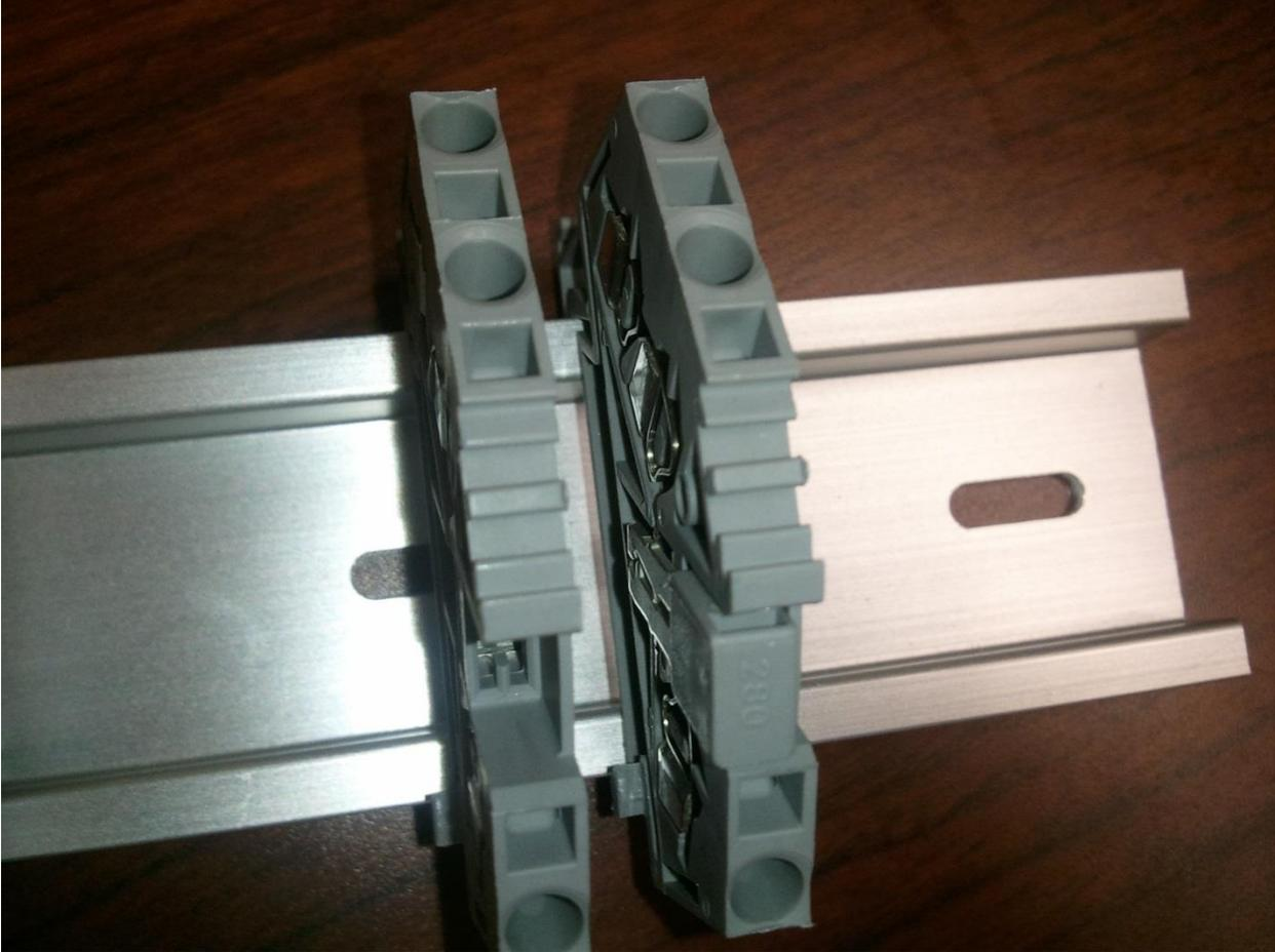
**Photograph 2.** Exaggeration of Improperly installed Jumper. Note the jumper cannot bridge the gap between the two DIN modules.
