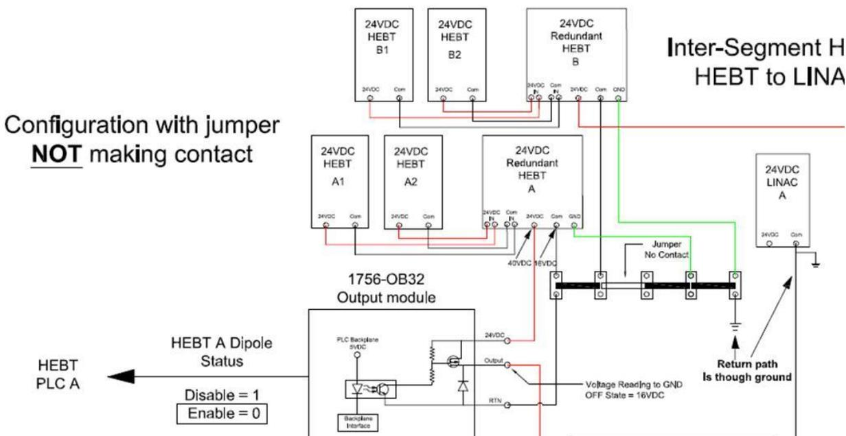
**Figure 1.** Schematic Depiction of PPS Redundant Power Supply Circuit
