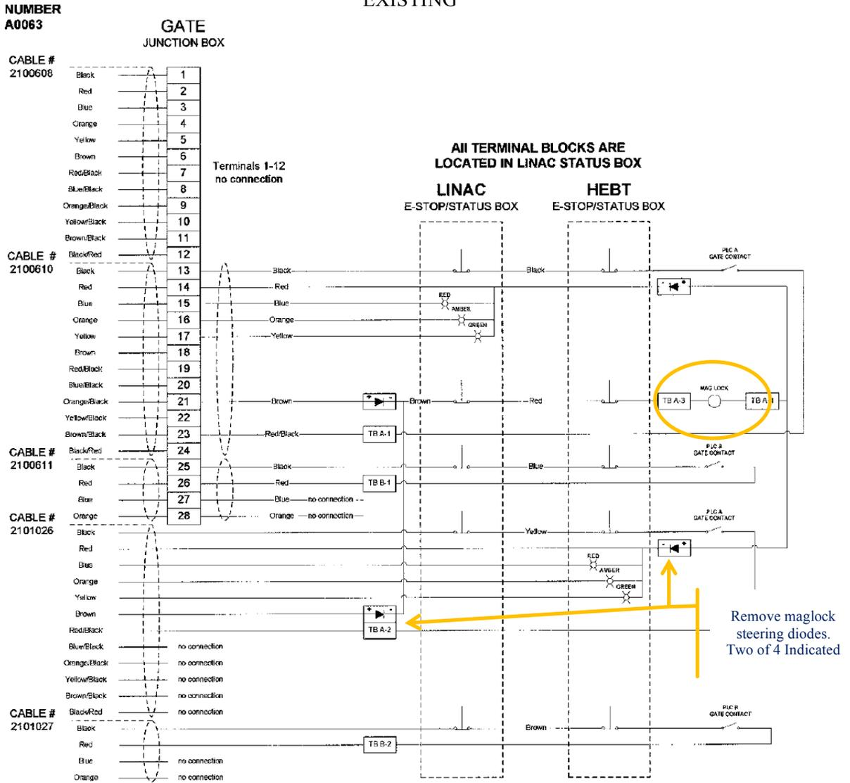
Figure 4 Existing gate maglock control using steering diodes
