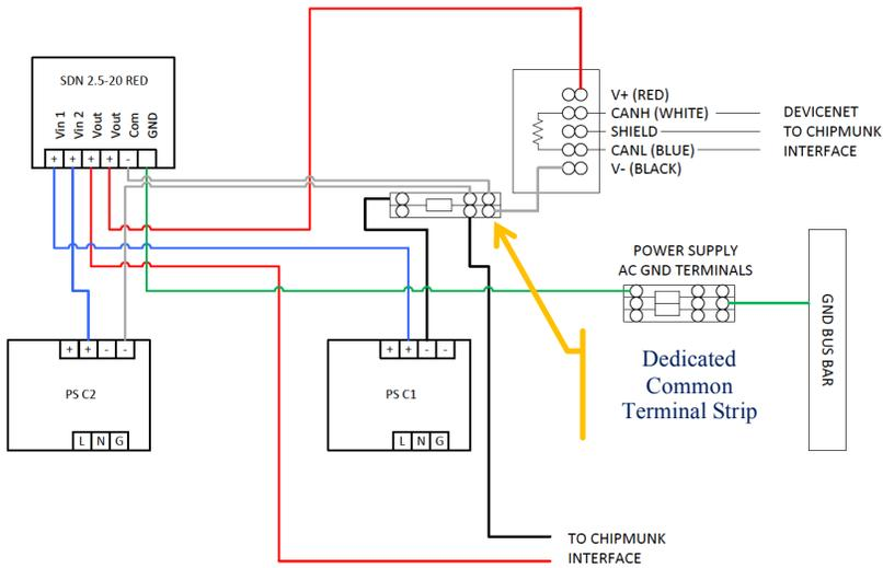
Figure 3 Existing and Proposed wiring of PLC 'C' Power in KL:CAB03
