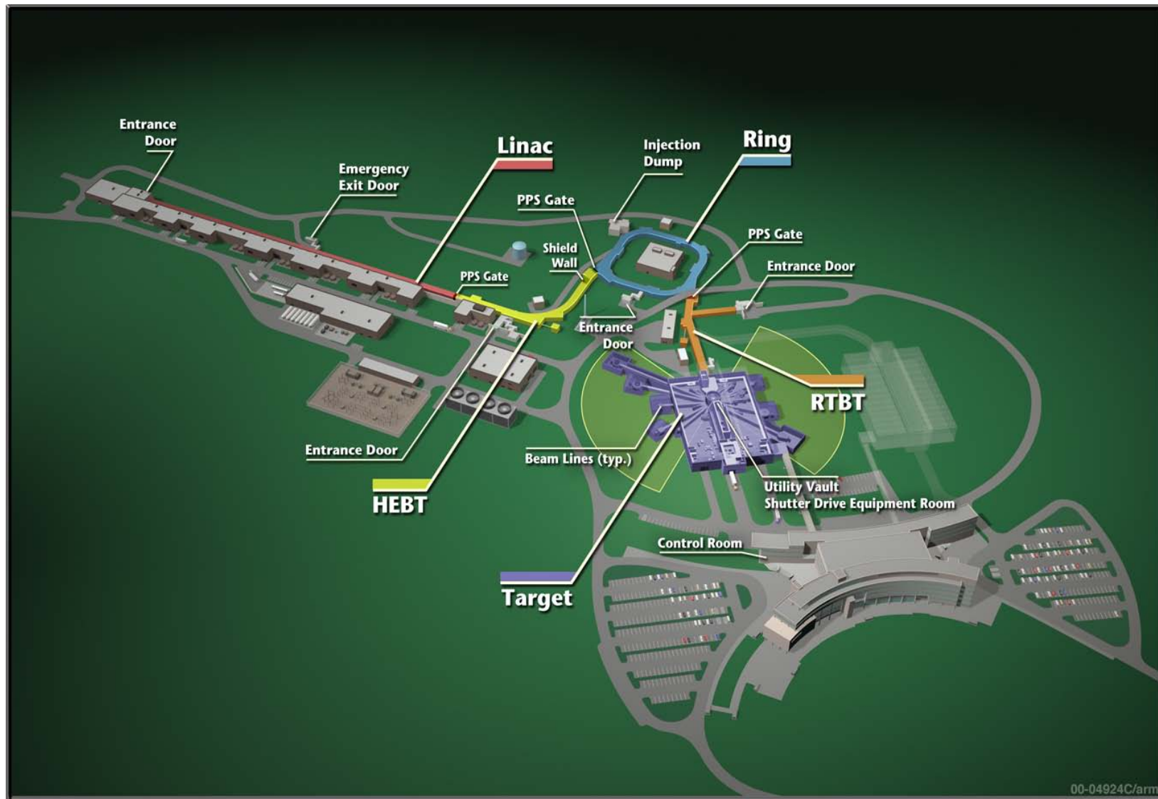
Figure 3.3.8.3.1-1 Overall Scope of the Personnel Protection System
