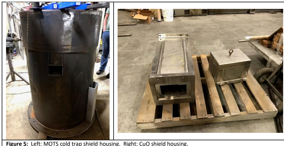
Figure 5: Left: MOTS cold trap shield housing. Right: CuO shield housing.
