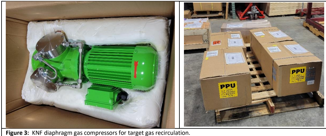
Figure 3: KNF diaphragm gas compressors for target gas recirculation.
