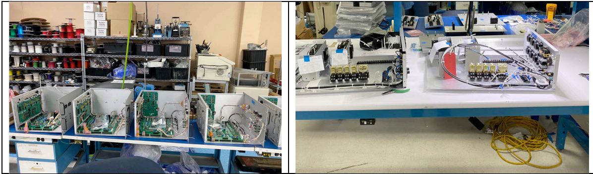
Figure 9: Main control chassis (left) and control power cassis fabrication (right).
