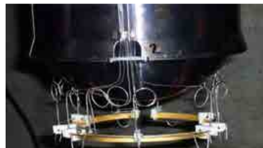
FIG. 4.65. MEGAPIE leak detector mounted at the beam entrance calotte of the liquid metal container.
