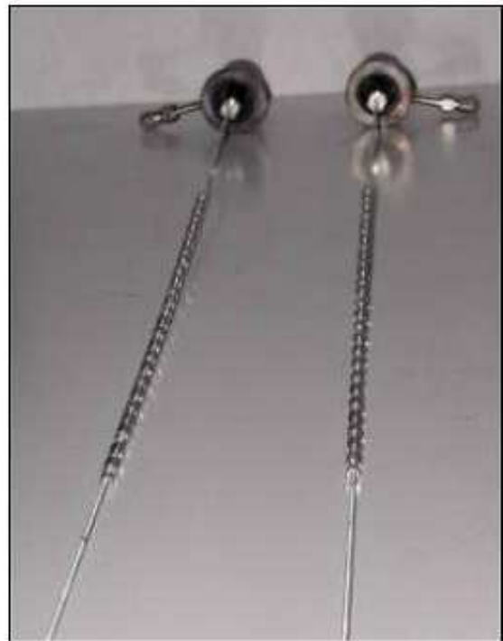
FIG. 4.34. Scheme of the test section and photo of the corrosion specimens before the tests.
