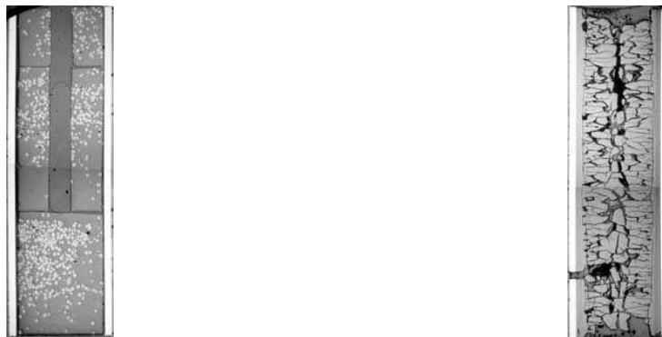
FIG. 4.94. Comparison of the microstructure of macrodispersed and microdispersed particle composites after irradiation: initial central hole remains in the macrodispersed sample (left side) where as it disappeared in the microdispersed sample (right side).
