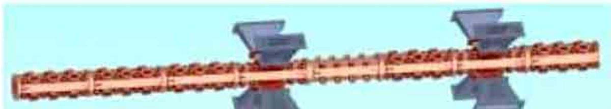
FIG. 3.20. Sketch of a 5MeV, 8 meters RFQ for the XADS LINAC.
