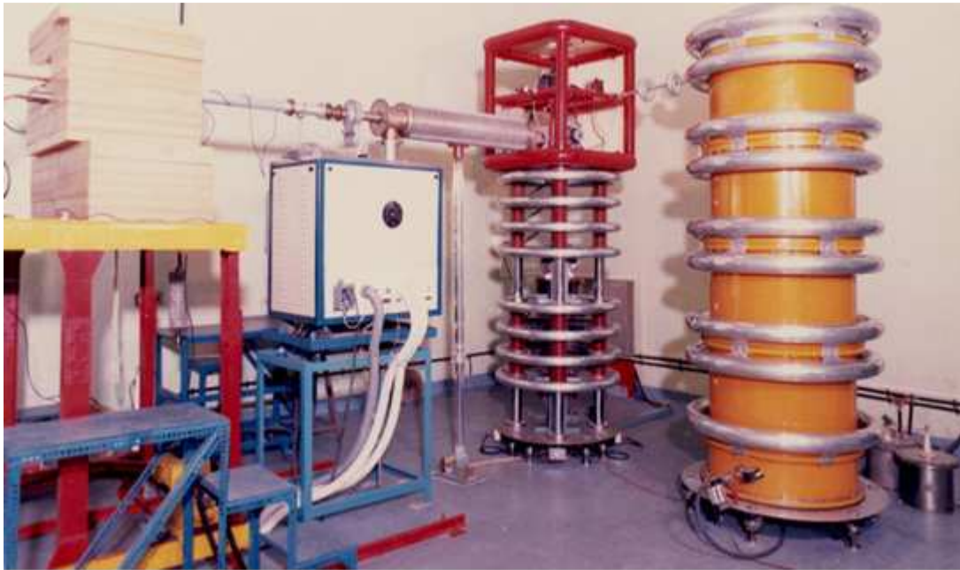
FIG. 4.10. 400 kV DC deuteron accelerator (right) for 14 MeV neutron source (on the left side).
