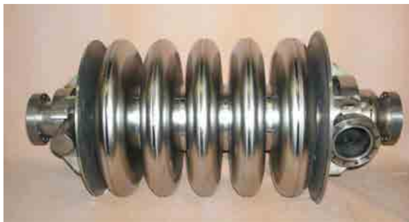
FIG. 3.23. 700 MHz, \beta=0.47 SC elliptical cavity prototype.
