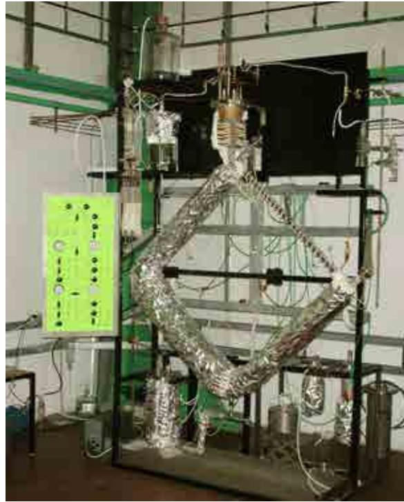
FIG. 4.13. Convection loop for corrosion tests in LBE COLONRI I.
