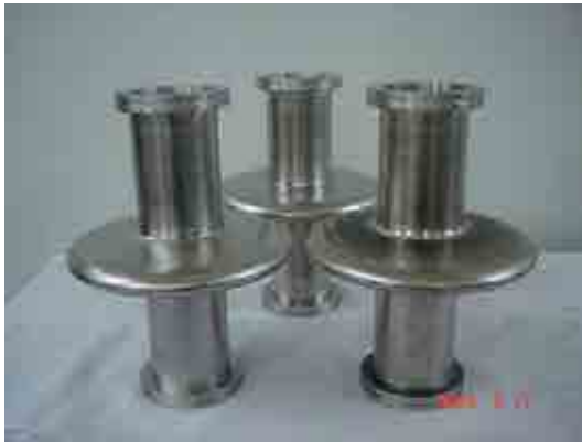
FIG. 4.40. 1.3 GHz, \beta=0.45 single cells.
