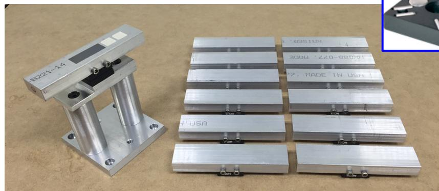
Thin-film substrate holders for GISAXS/GIWAXS (~10 substrates per holder)
