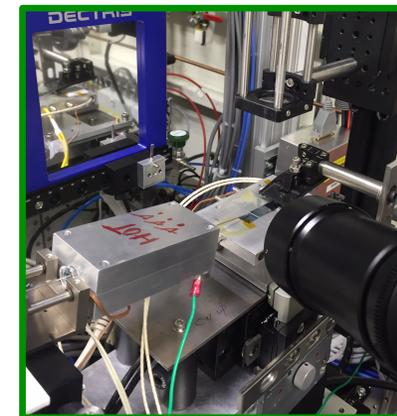
Blade coater for thin film fabrication and annealing
