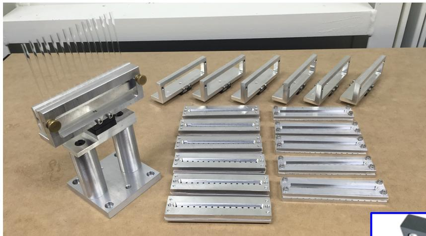
Sample holders for transmission SAXS/WAXS (15 positions per holder)
