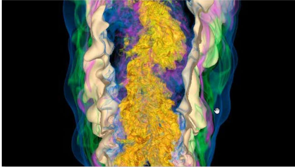
A visualization of the mixture fraction isosurface (gold) and HO_2 , which shows autoignition occurring in fuel-lean mixtures at regions with high temperatures, low mixing rates, and short ignition delay times. Image credit: Hongfeng Yu, University of Nebraska; and Kwan-Liu Ma, University of California, Davis
