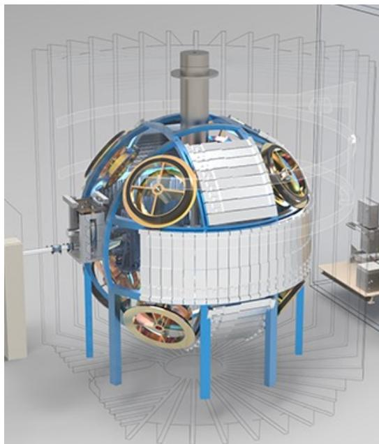
CHESs, a direct geometry neutron spectrometer.
