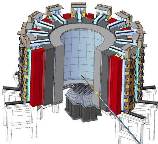
PIONEER, a high Q-resolution polarized single-crystal neutron diffractometer.
