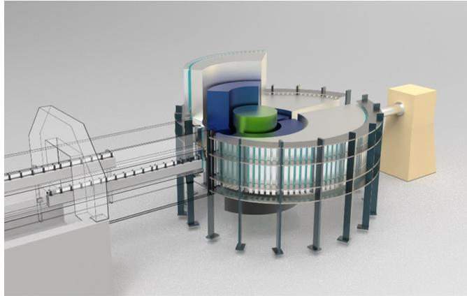
VERDI: VERsatile Diffractometer with wide-angle polarization analysis for magnetic structure studies in powders and single crystals
