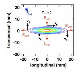
$\text{Lorentz force: } \vec{F} = q \cdot (\vec{v} \times \vec{B}_{ext} + \vec{E}_{self}) \qquad \text{Drift: } \vec{v}_E = \frac{\vec{E}_{self} \times \vec{B}_{ext}}{B_{ext}^2}$
