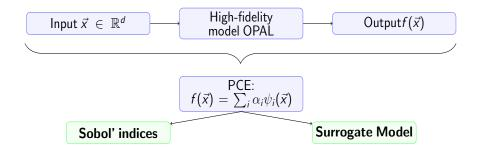
Allows for fast multi-objective optimization.
