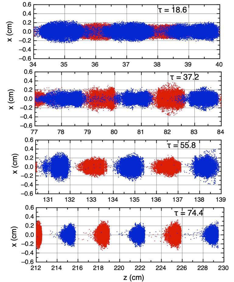
Formation of the two-component beam in RFQ: (red) H<sup>+</sup> beam, (blue) H<sup>-</sup> beam.
