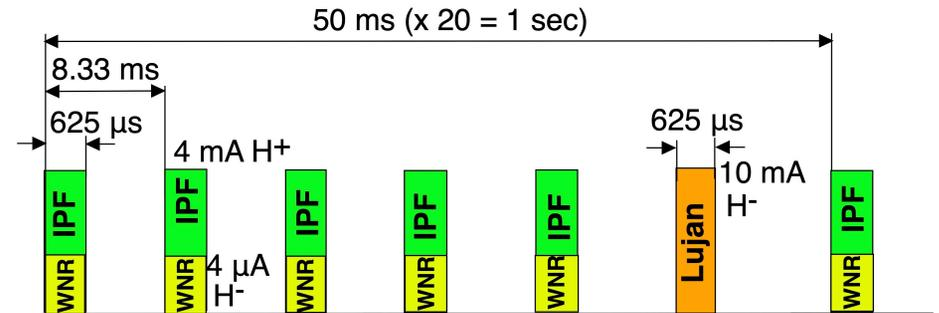
Layout of Lujan/WNR/IPF beams. Beams delivered to pRad or UCN facilities “steal” their time cycles from WNR beam.
