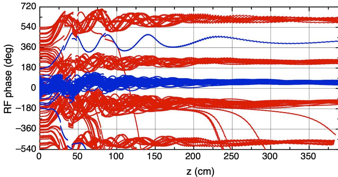
Phase trajectories in RFQ: (red) H<sup>+</sup> beam, (blue) H<sup>-</sup> single bunch beam.
