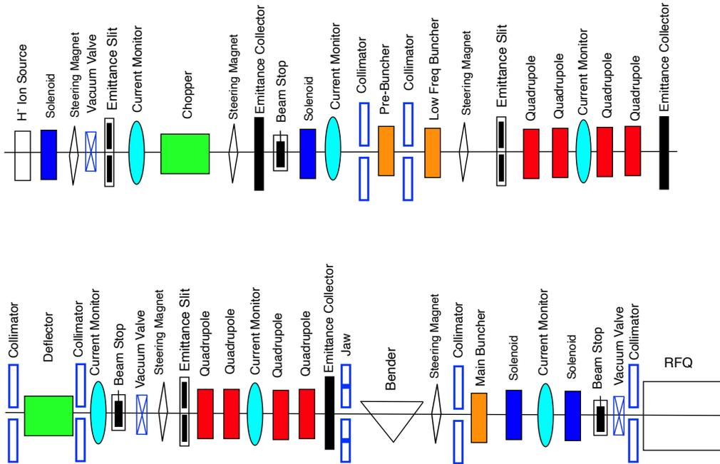
Layout of H<sup>-</sup> leg of injector part with additional beamline elements.
