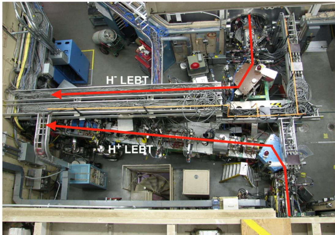
Top view of existing 750 - keV Low Energy Beam Transports (LEBT) of  $H^+$  and  $H^-$  beams.
