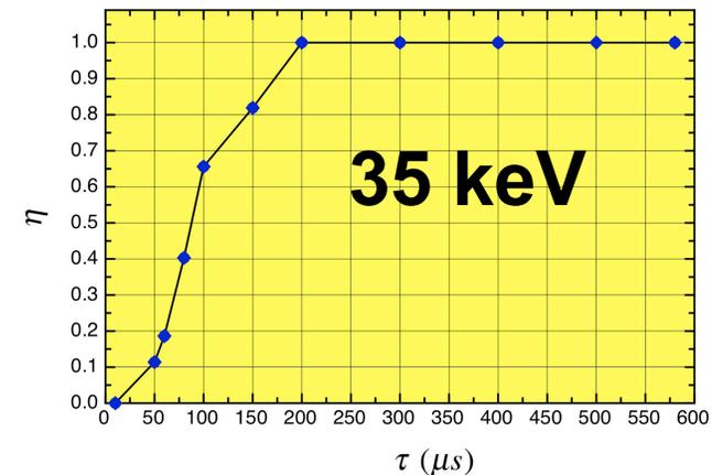
Space charge neutralization of H<sup>-</sup> beam as a function of beam pulse length (Y.B. et al, IPAC13, TUPWA066).
