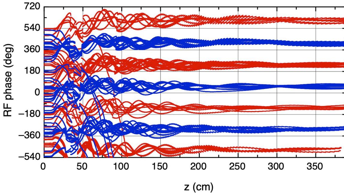
Phase trajectories in RFQ: (red) H<sup>+</sup> beam, (blue) H<sup>-</sup> beam.
