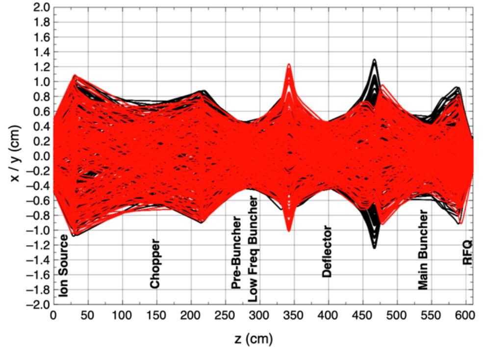
Particle trajectories in the Low-Energy Beam Transport: (red) horizontal, (black) vertical.
