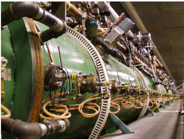
100 MeV Drift Tube Linac
