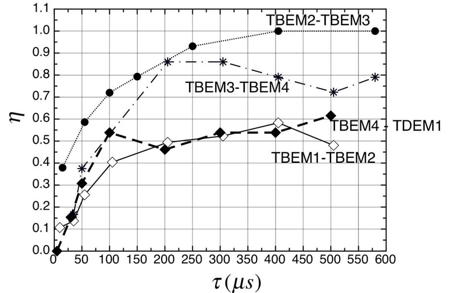
Space charge neutralization of H<sup>-</sup> beam as a function of beam pulse length (Y.B., NIM-A 904 (2018) 64-73).
