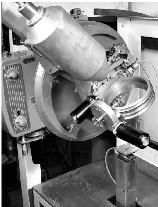
Bill Busing, Hal Smith, Pete Peterson, Henri Levy, automatic three-circle neutron diffractometer 1961
