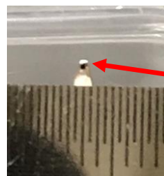
μg single crystals can be measured on WAND 2
