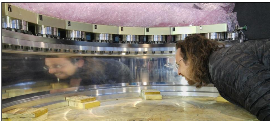
μg single crystals can be measured on WAND 2
