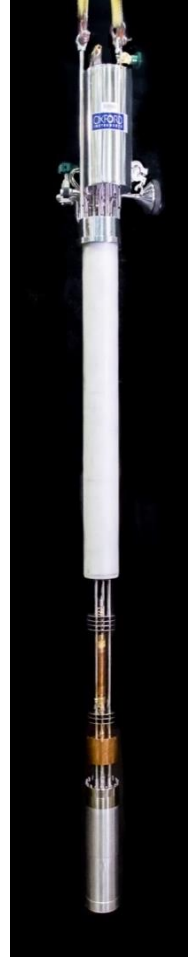
3 He insert 300 mK – 300K or Dilfridge insert 100 mK – 300K
