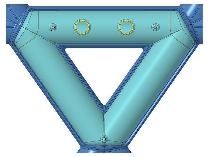
Vacuum vessel body opening designed to just allow the hydrogen vessel to fit for assembly
