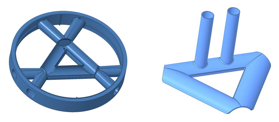
Machined from single forgings – vacuum vessel body pushes machining complexity limit
