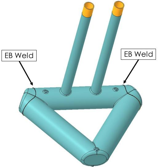
Constant 2 mm weld thickness welded in 2 passes with simple weld geometry
