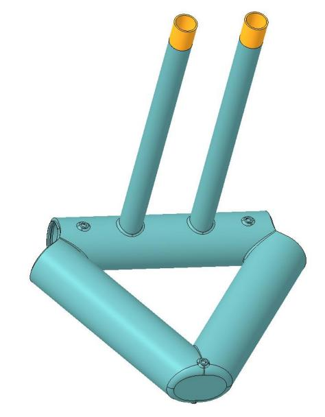
Interface features and majority of hydrogen boundary integrated into single part
