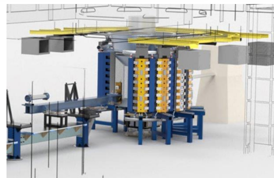
PIONEER diffractometer optimized for small samples
