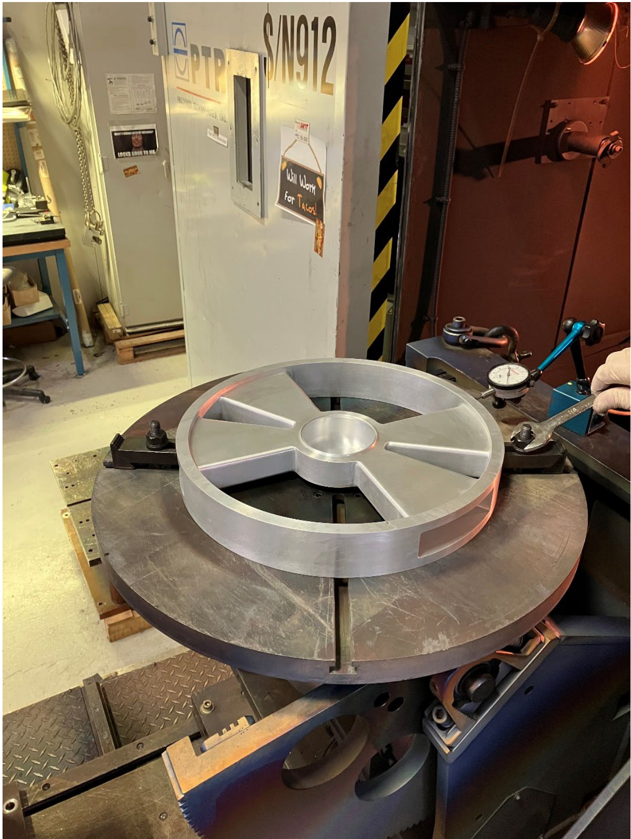
Vacuum vessel body being indicated in on rotary table.
