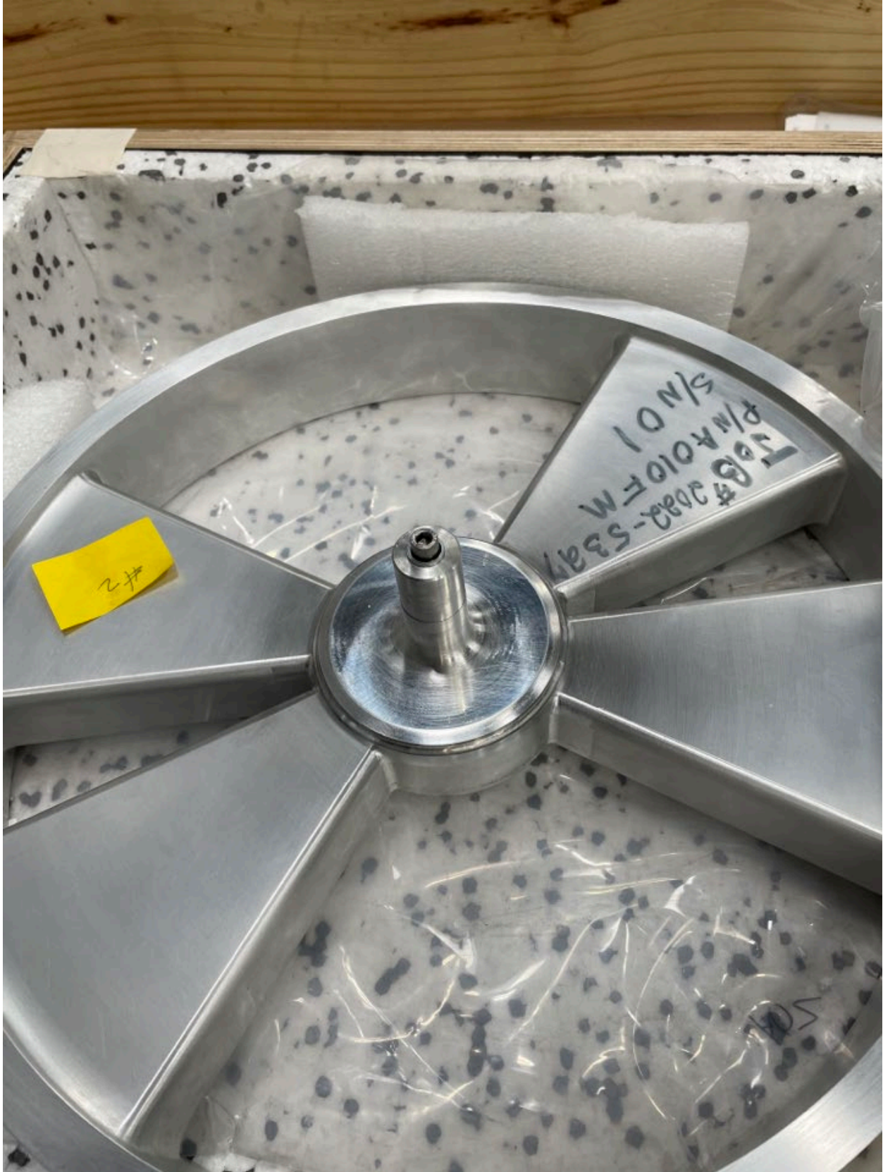
Vacuum vessel after post weld machining completed at Metalex.
