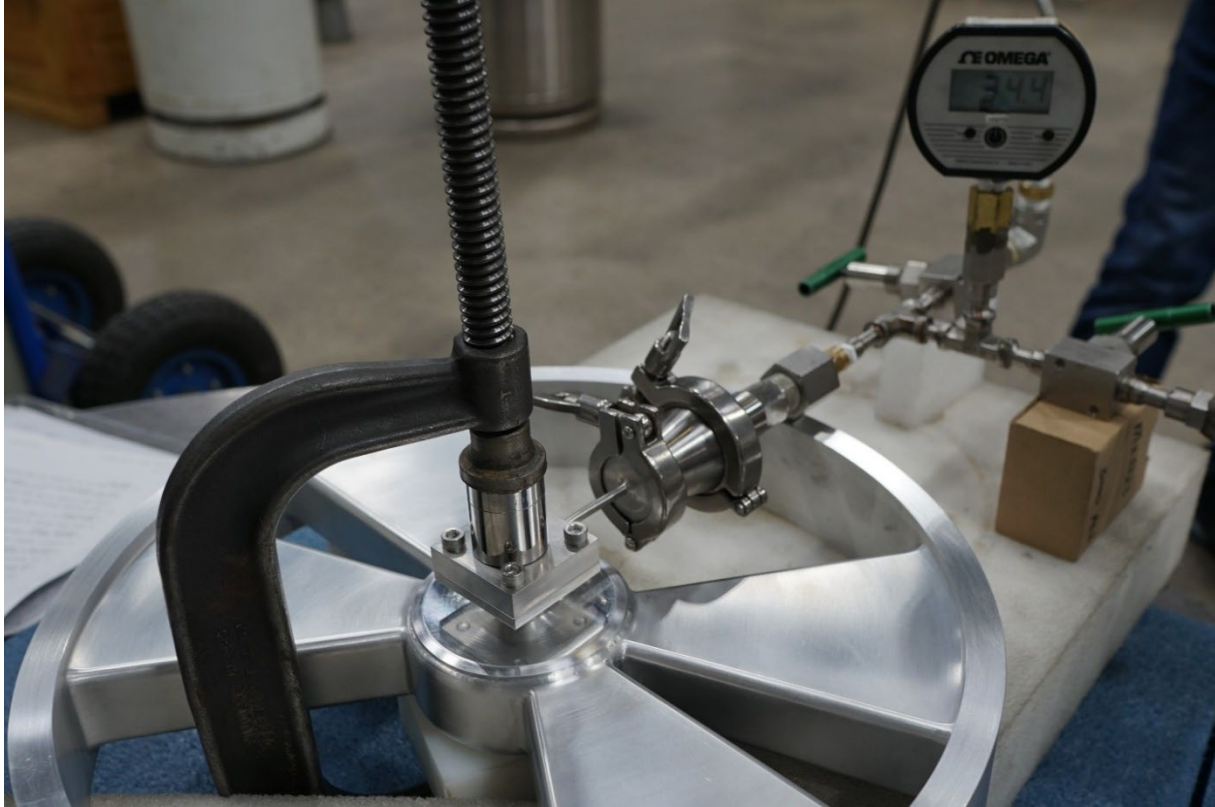
Vacuum vessel pressure test at test pressure.
