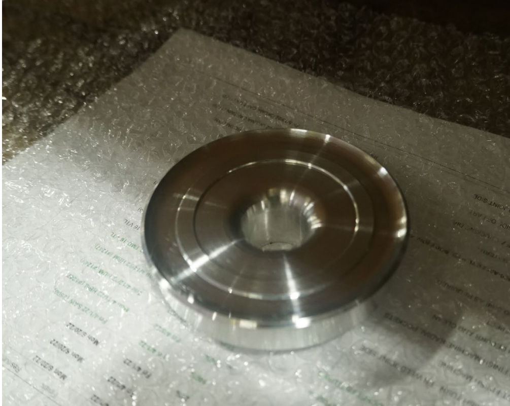
Vacuum vessel lid finished with lathe work and ready for milling of pockets.
