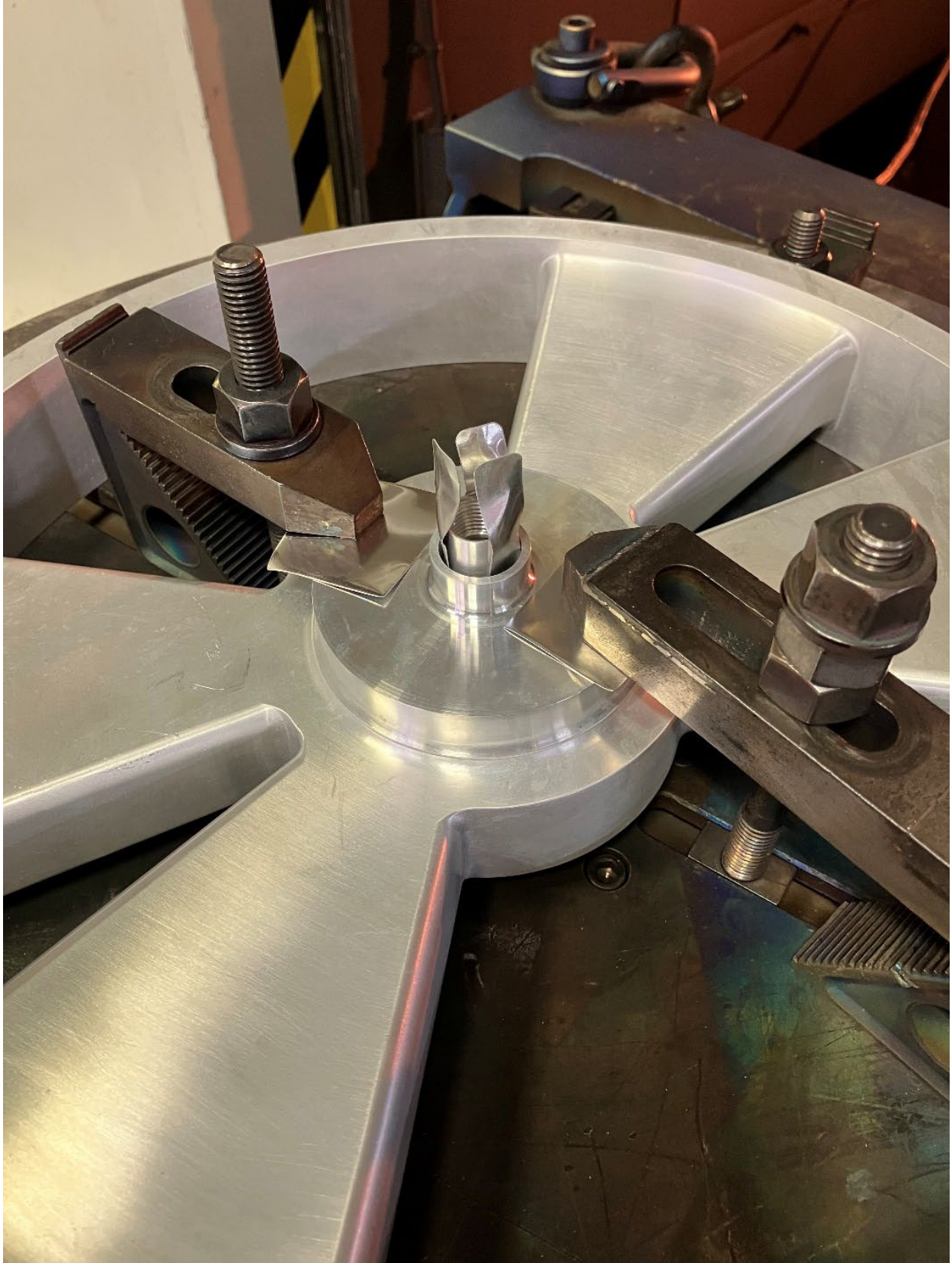
Vacuum vessel lid installed and clamped down for tacking.
