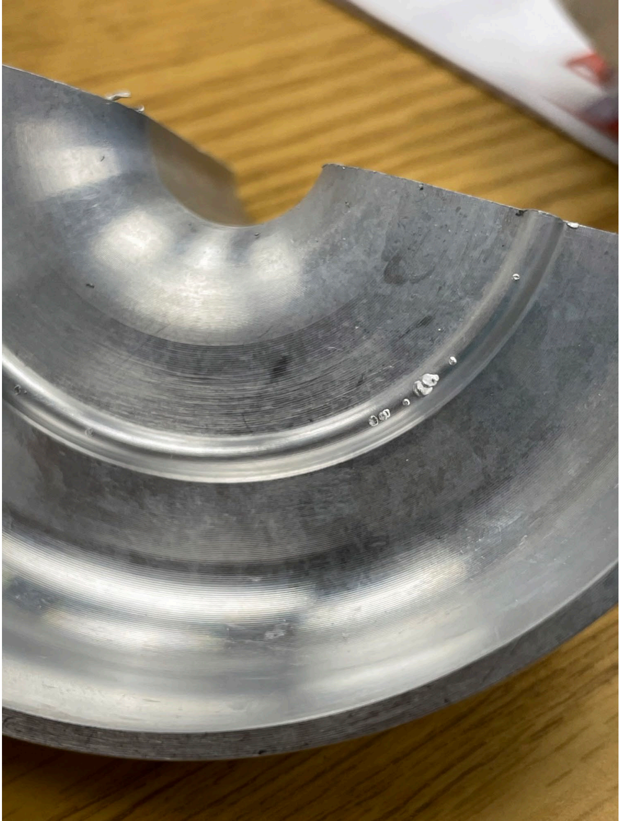
Intermittent over penetration of hydrogen vessel sample weld.
