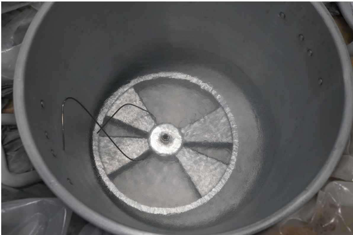
Cold shocking in LN2 at Metalex.
