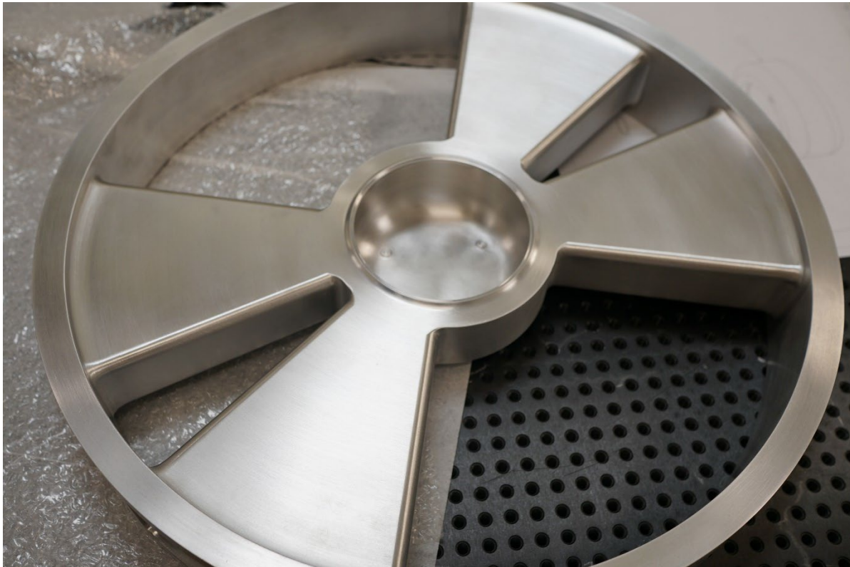
Vacuum vessel body at receipt.
