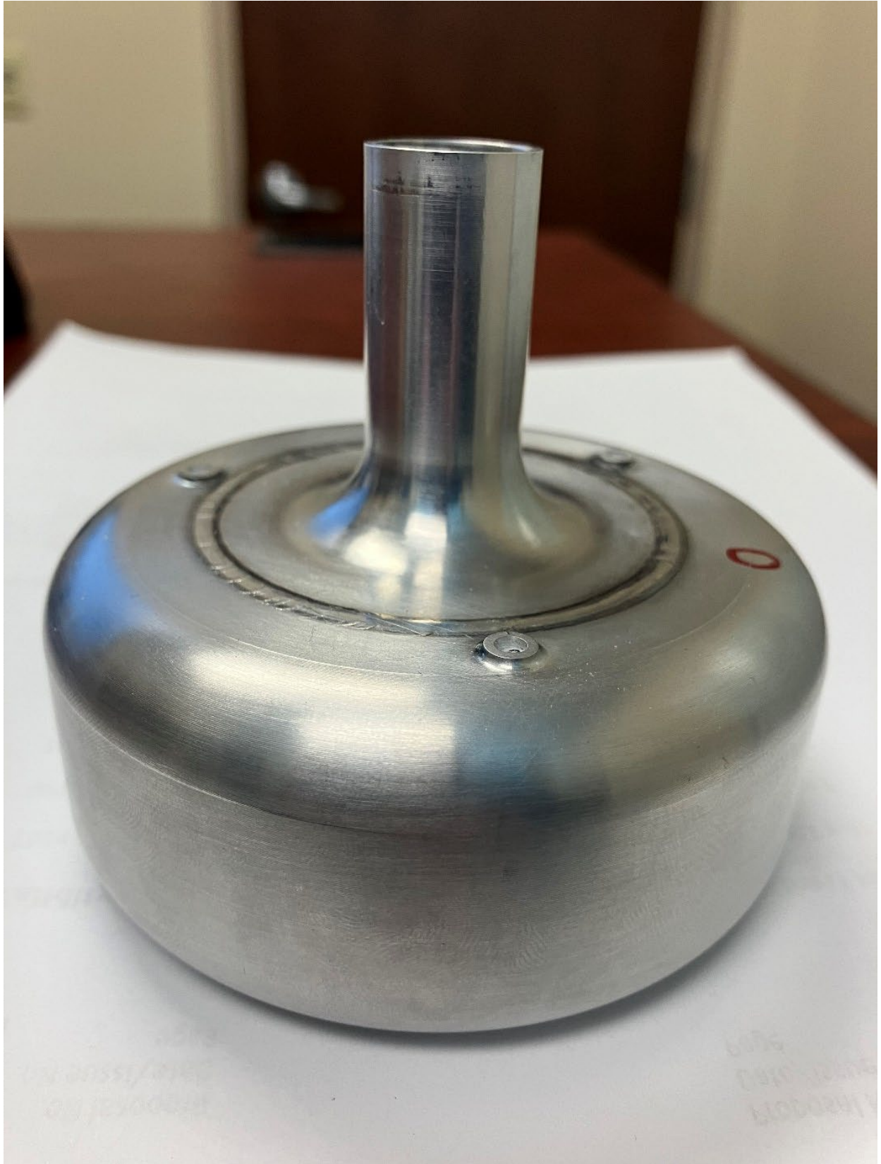
Completed hydrogen vessel.
