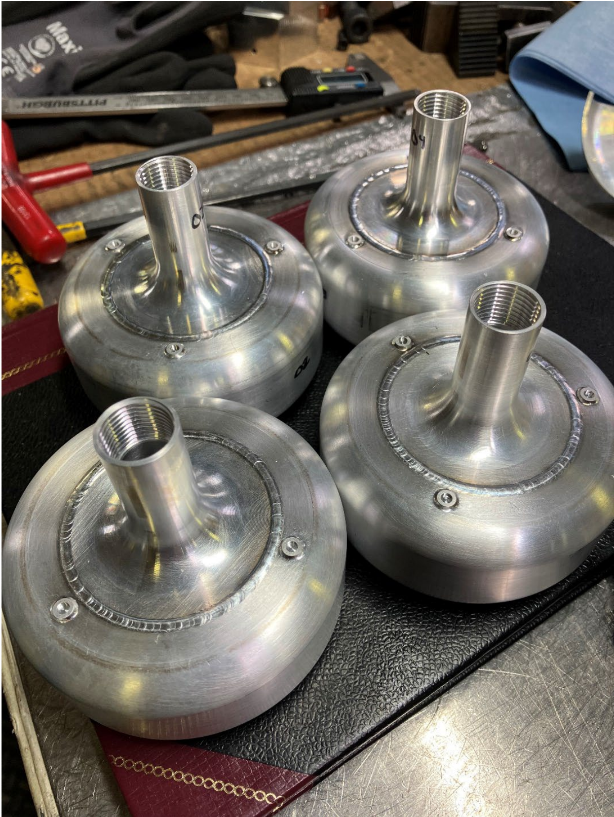
Four completed hydrogen vessels.
