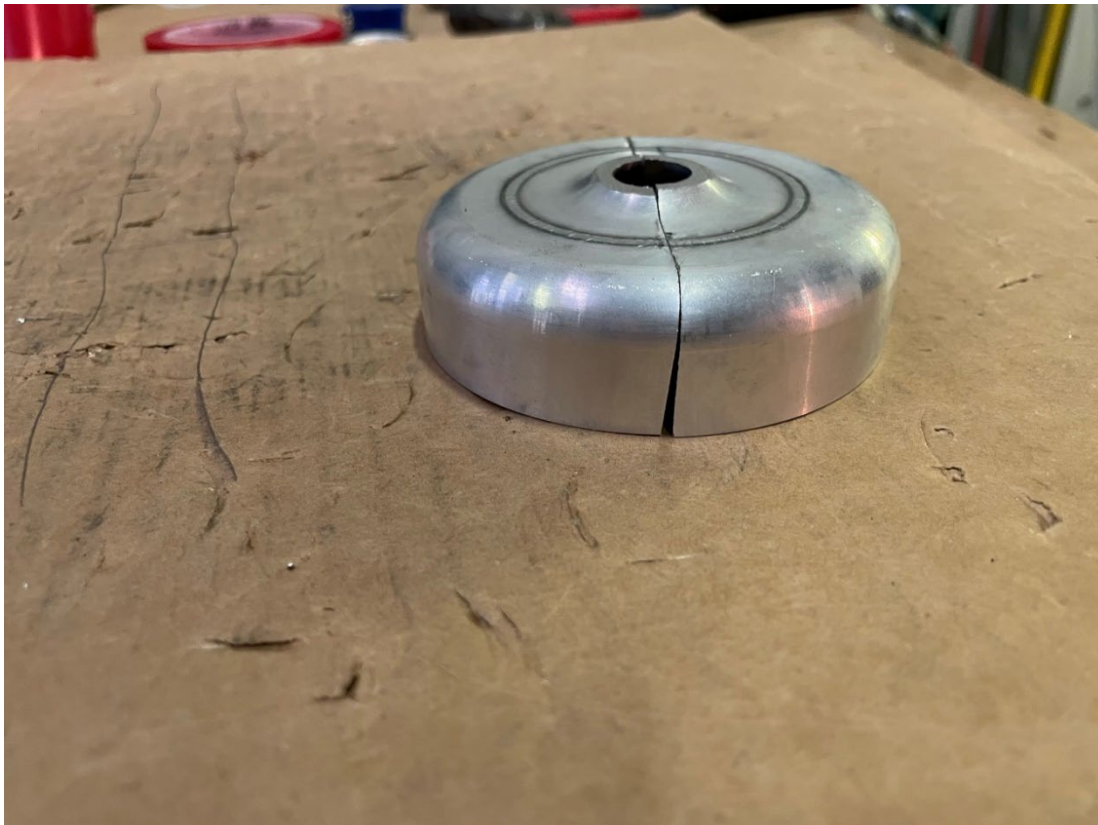
Beam strikes on the hydrogen vessel sample due to overpenetration of the vacuum vessel weld.
