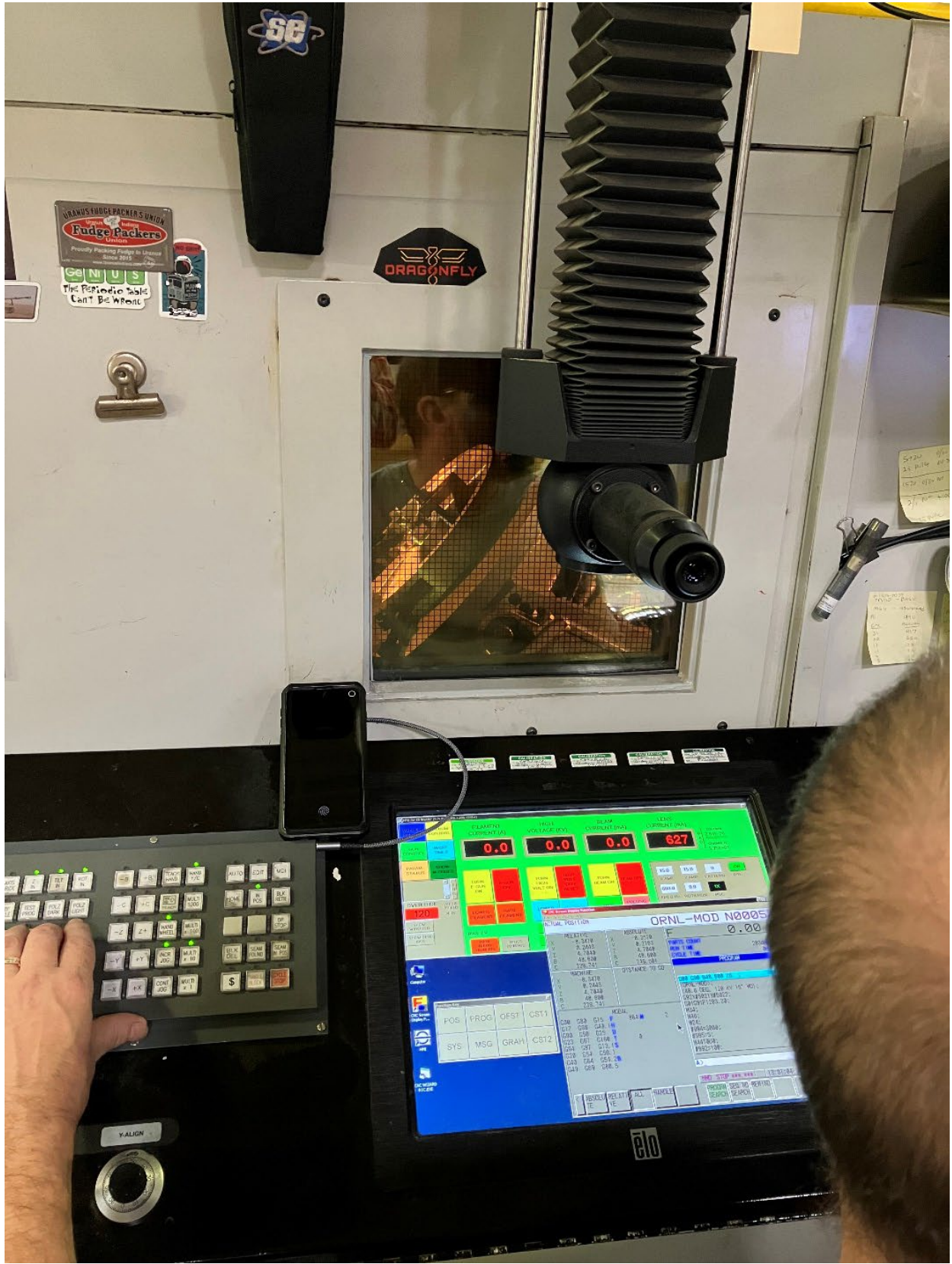
Vacuum vessel welding in the EB weld chamber.
