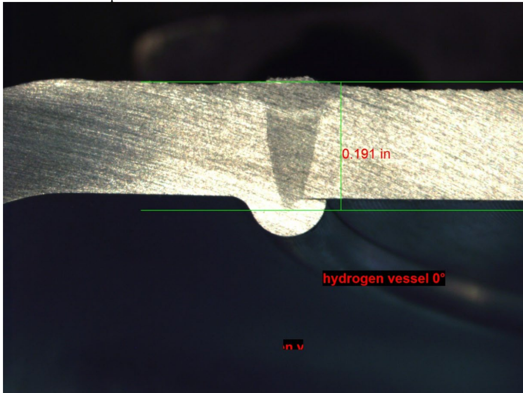
Hydrogen vessel weld section at start of weld.
