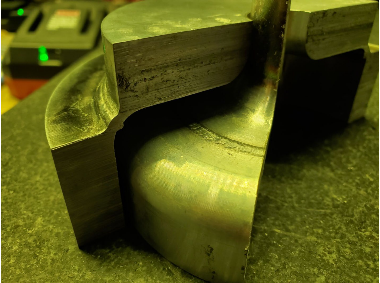
Already welded sample hydrogen vessels were placed inside sample vacuum vessel welds during welding to determine the effect of overpenetration.
