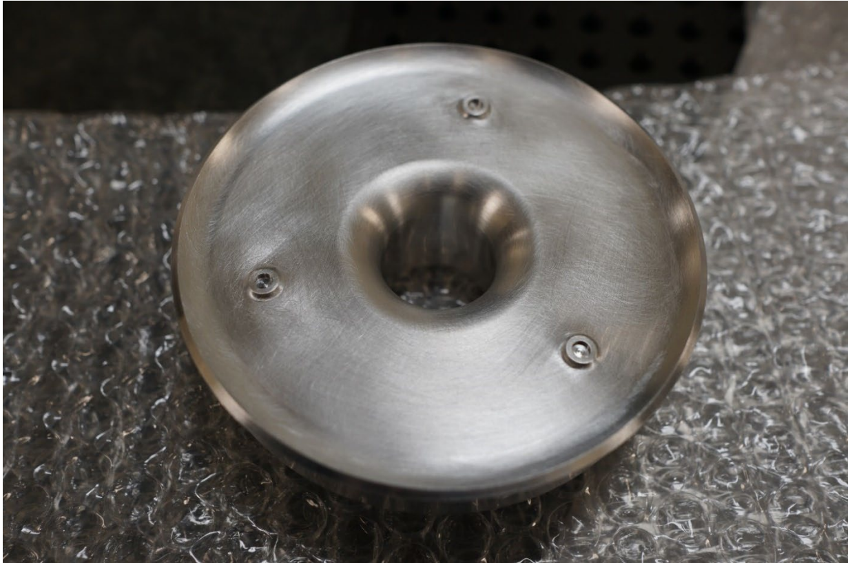
Vacuum vessel lid at receipt.
