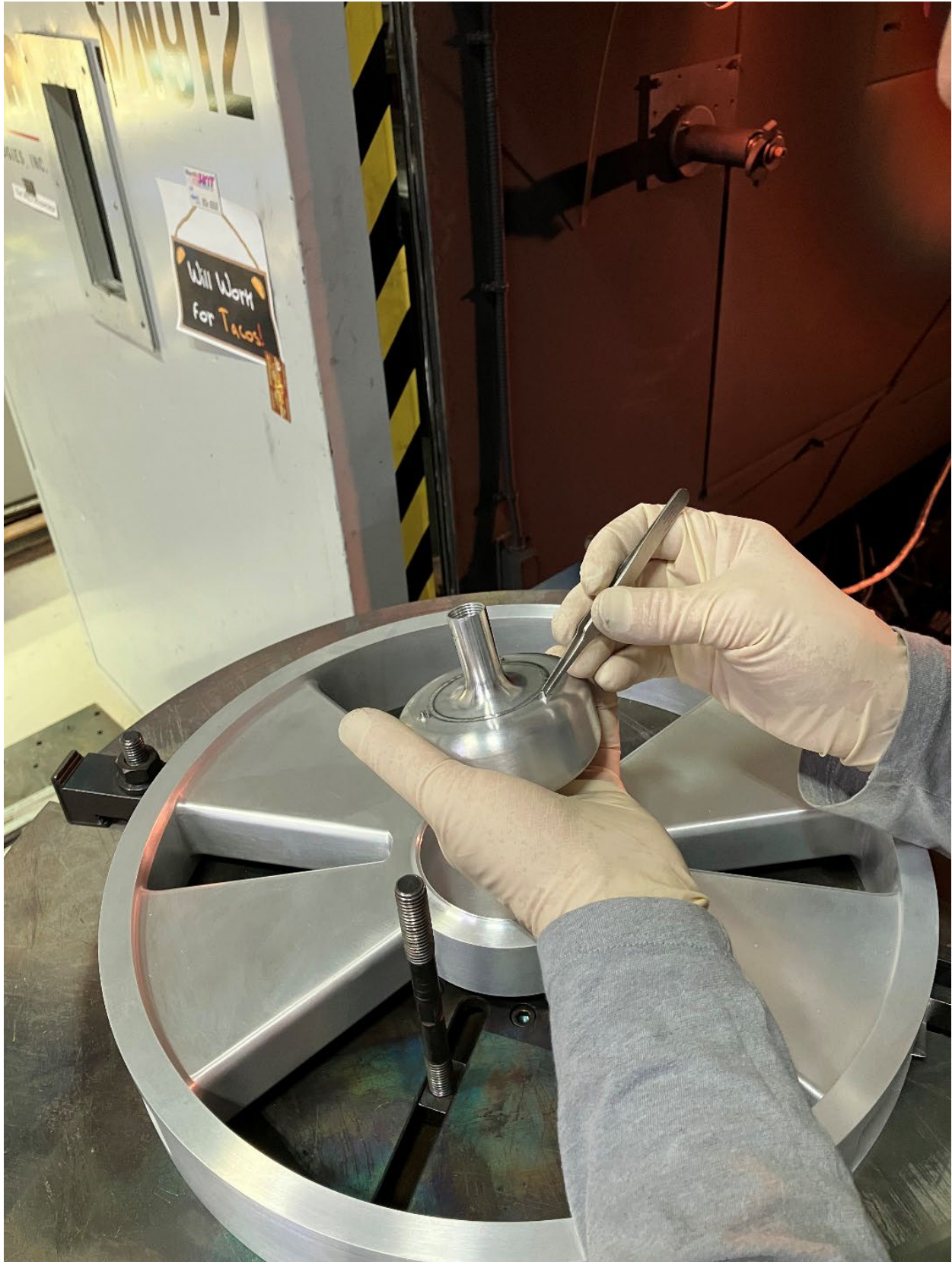
Tedious installation of titanium spacers onto hydrogen vessel.
