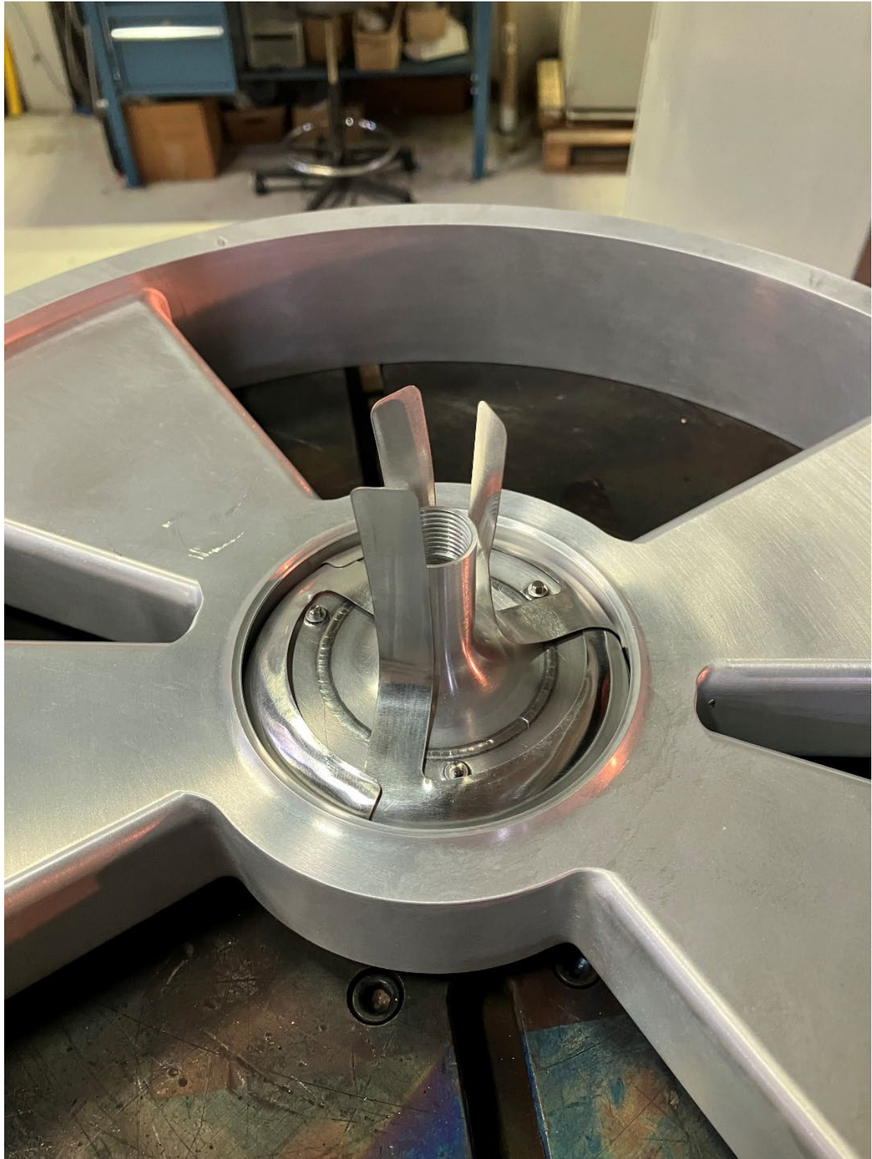
Hydrogen vessel with beam blocker shims installed into vacuum vessel body.
