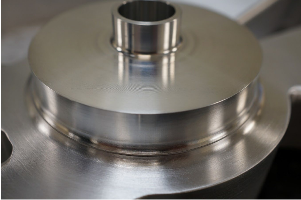
Testing fit up of vacuum vessel body to lid at receipt.
