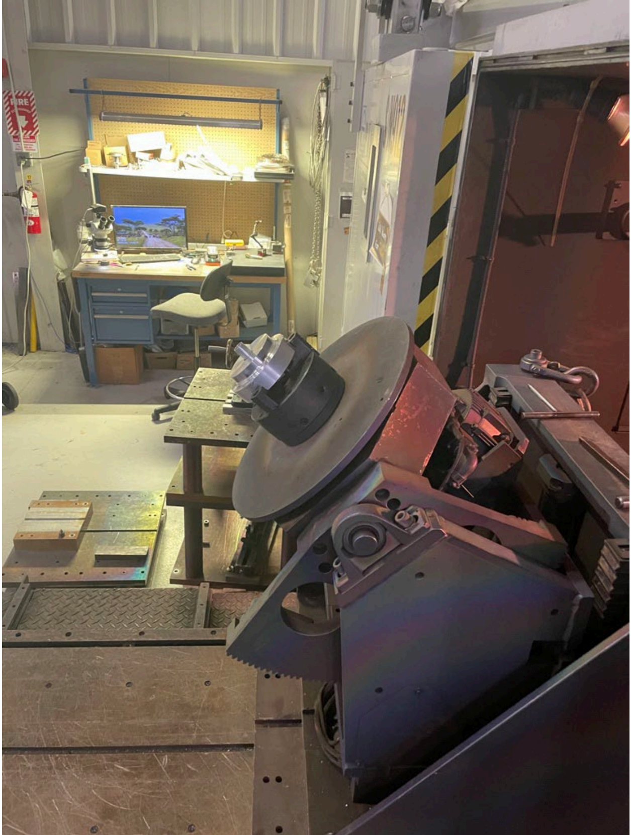
Loading vacuum vessel weld sample into EB weld machine.
