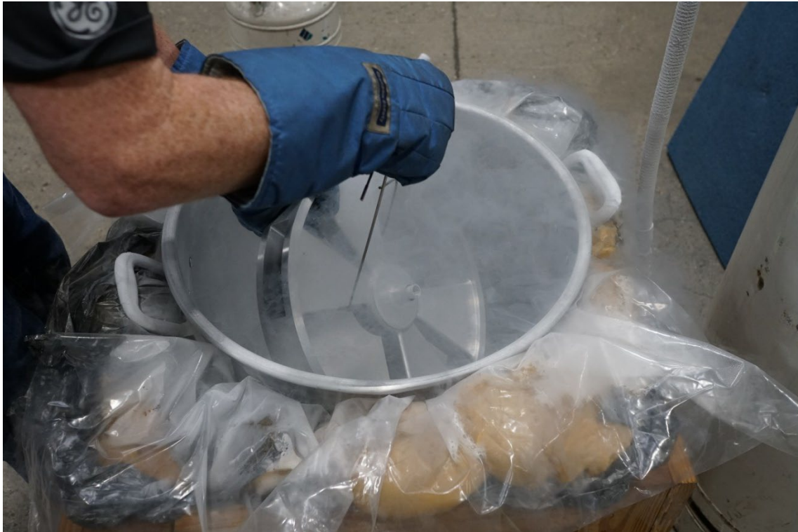
Cold shocking in LN2 at Metalex.
