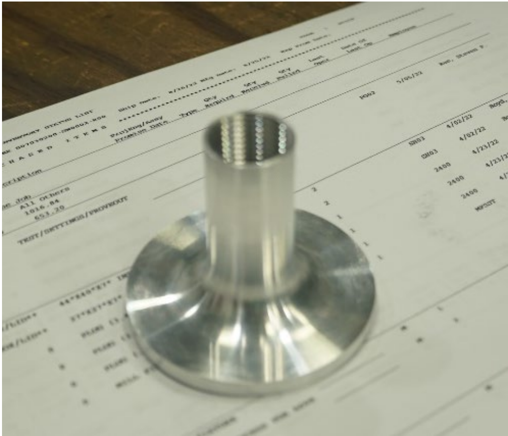
Finished hydrogen vessel lid.
