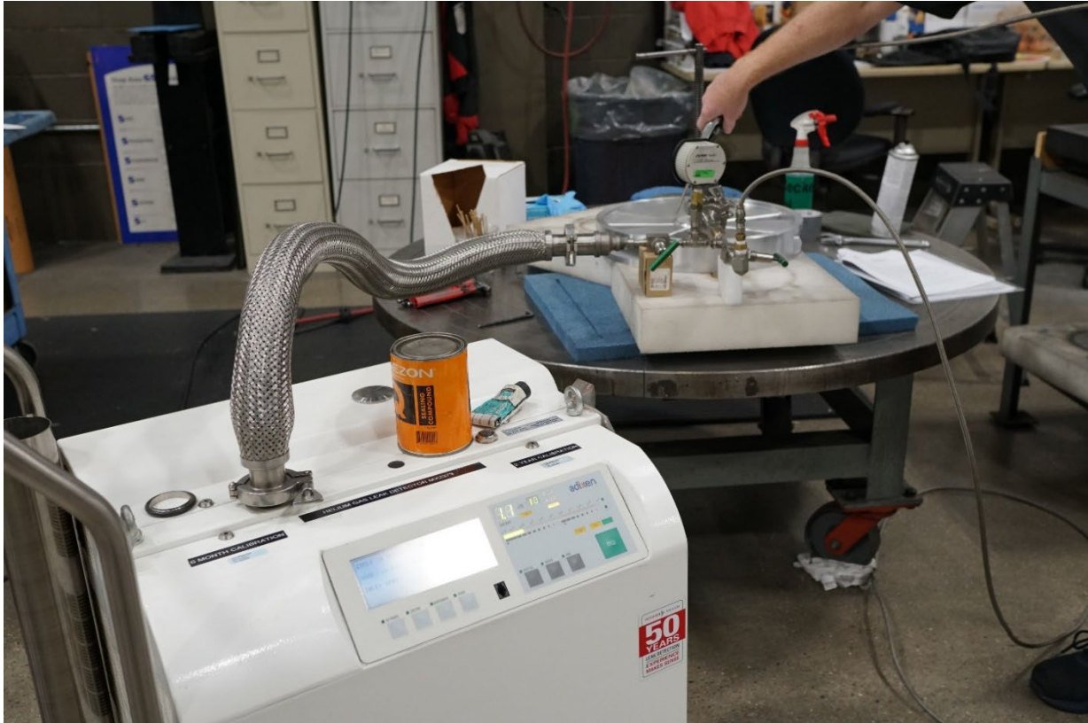
Vacuum vessel leak checking at Metalex.
