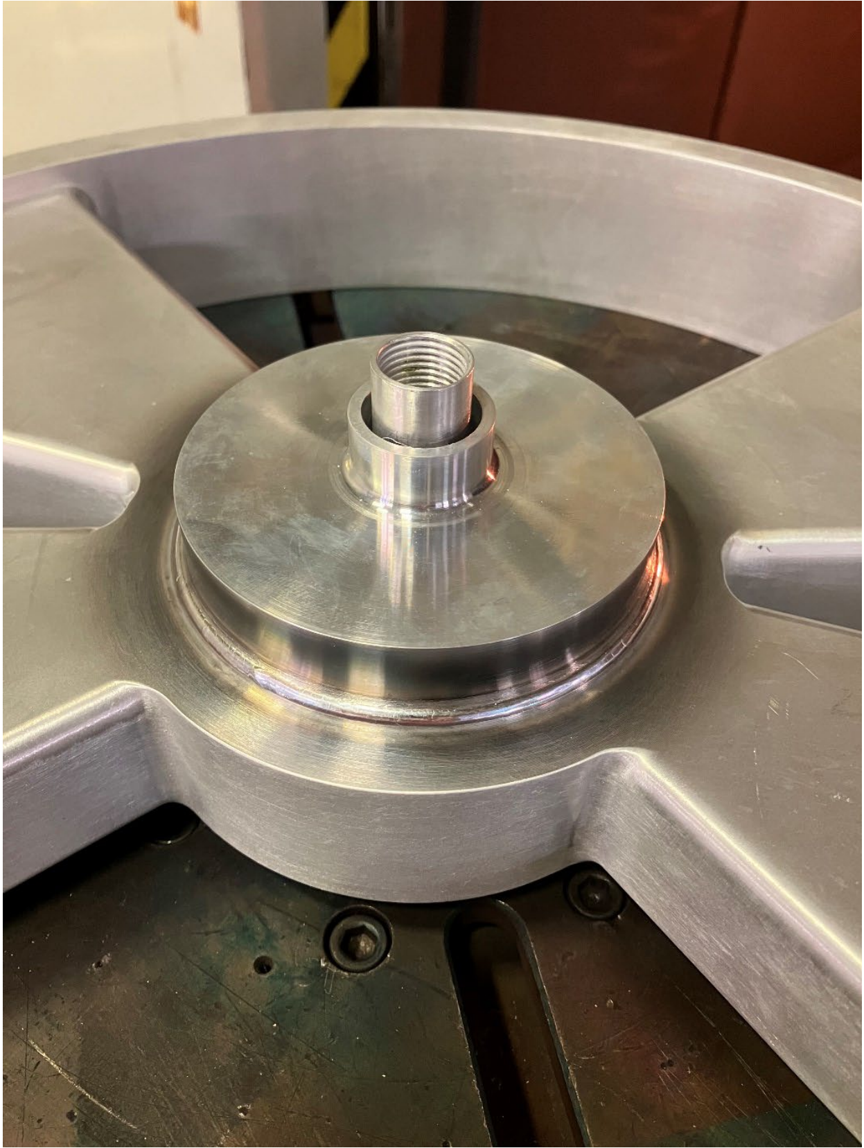
Vacuum vessel weld completed and shims unsuccessfully removed (broken off at lip).
