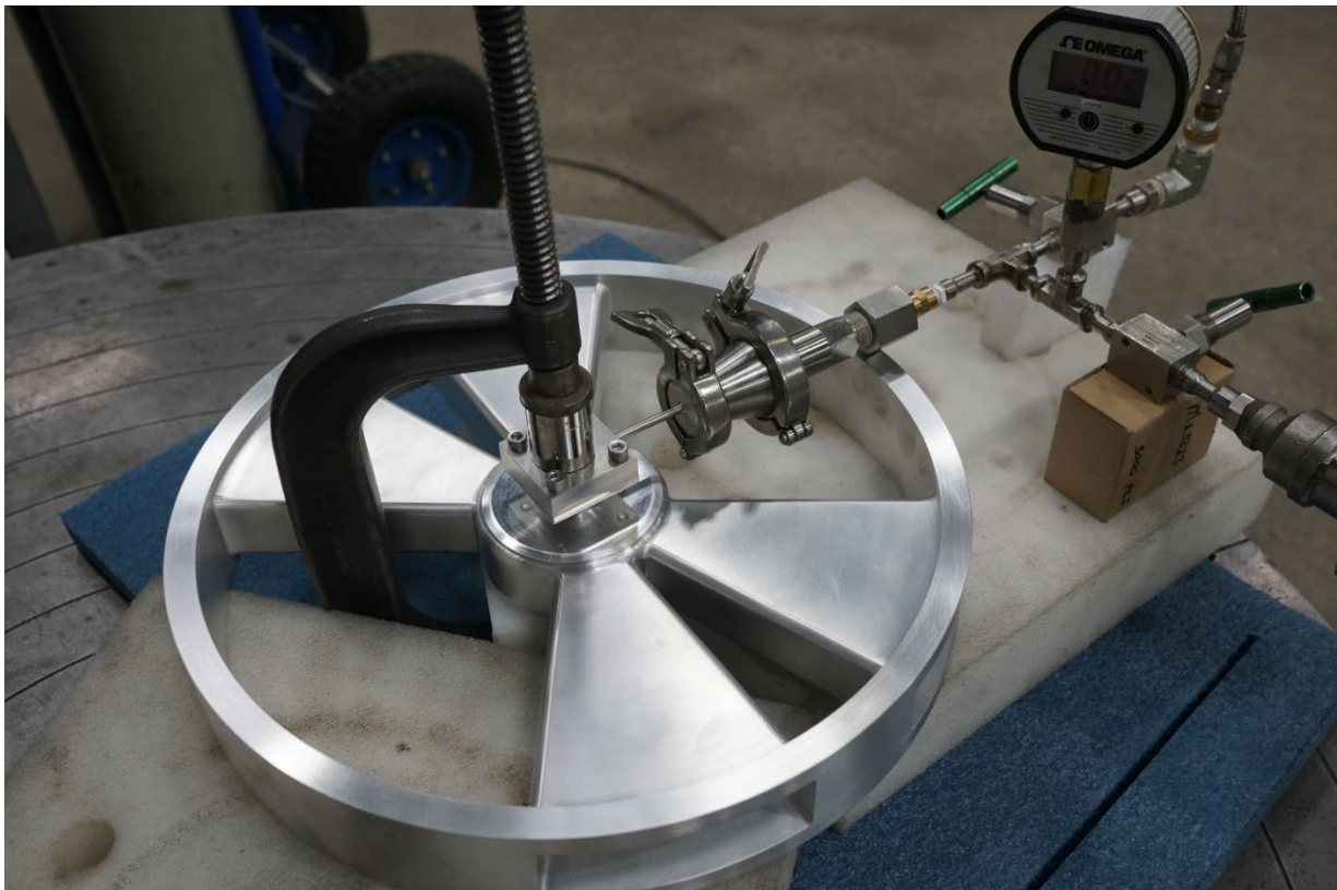
Vacuum vessel pressure testing set up.
