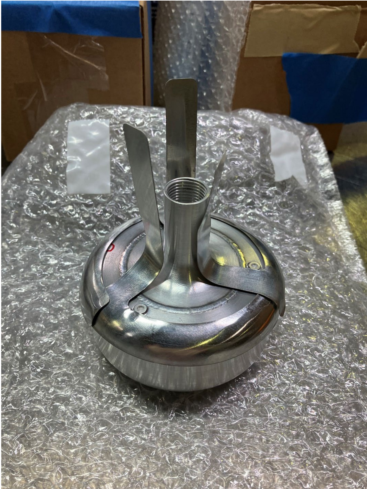
Hydrogen vessel with beam blocker shims installed.
