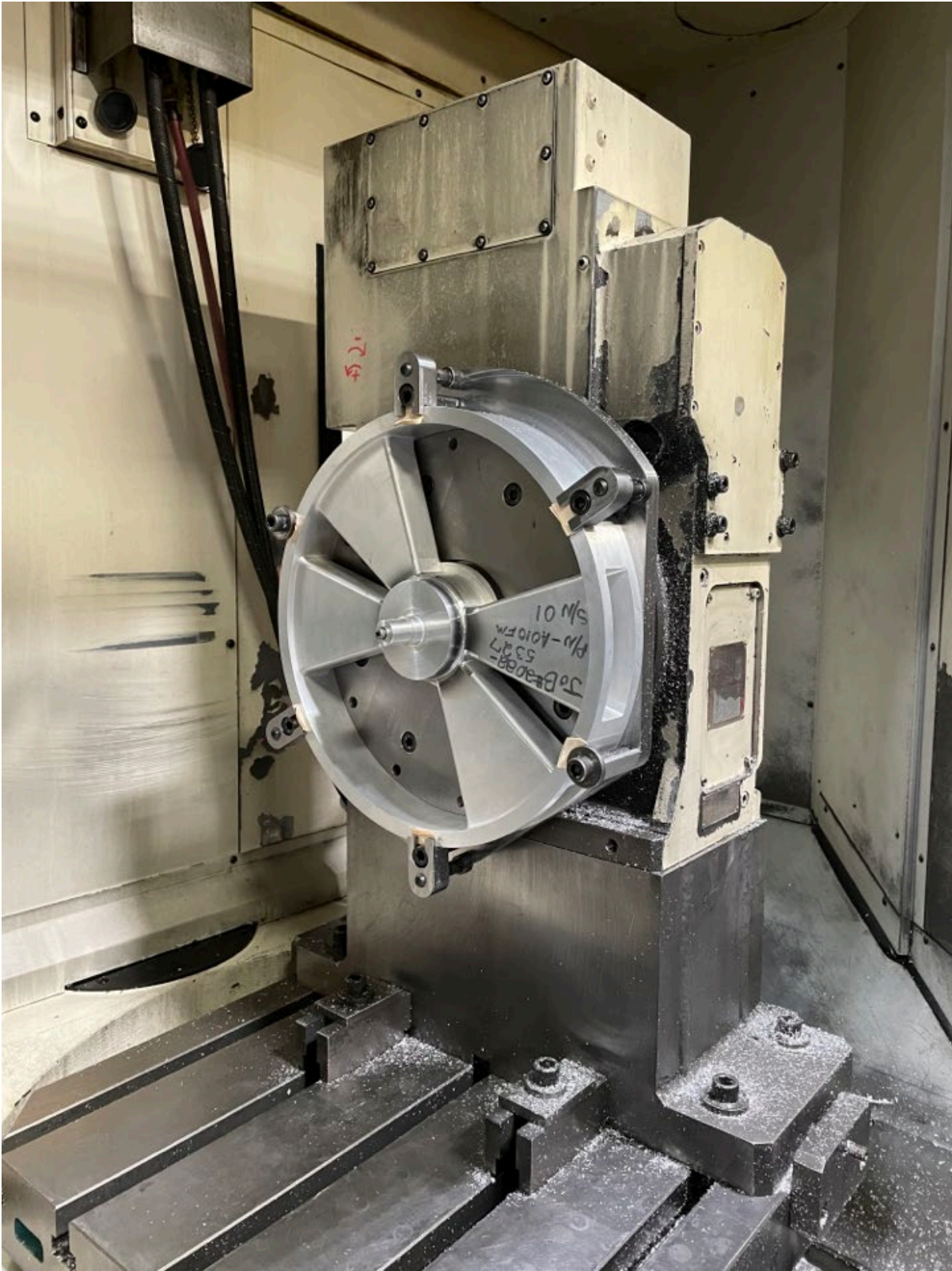
Vacuum vessel undergoing post weld machining at Metalex.
