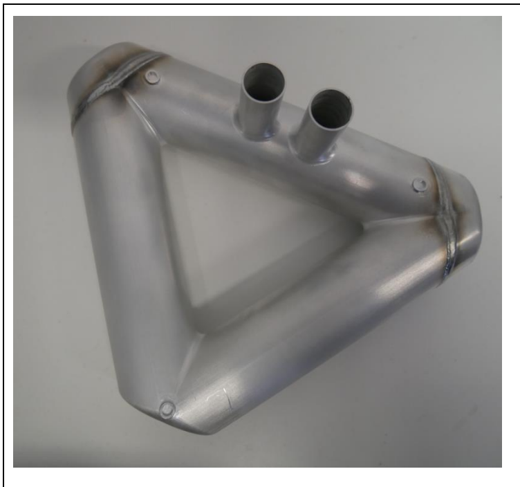
Figure 4.3: Hydrogen vessel after the final welding
