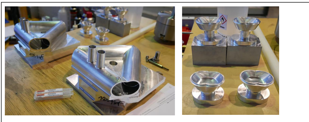
Figure 3.2: Machined parts of the hydrogen vessel and end caps
