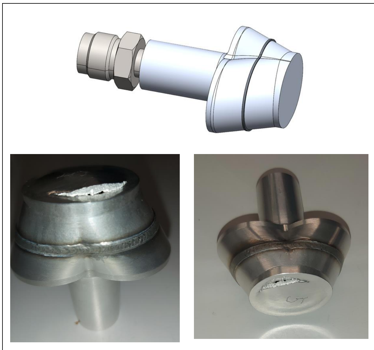
Figure 5.31: Hydrogen vessel welding sample - water burst test
