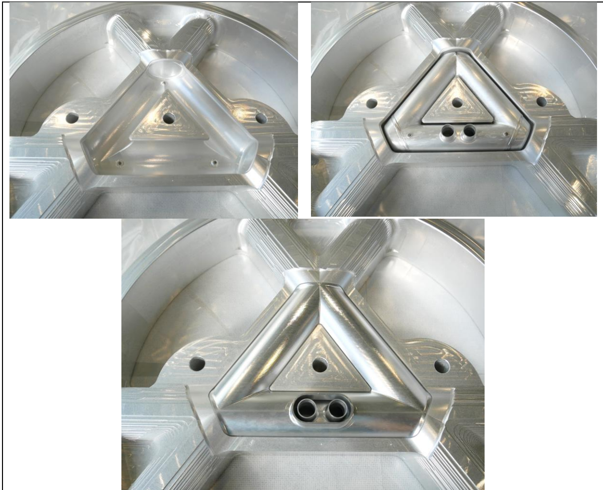
Figure 3.11: Assembly of the vacuum vessel with the hydrogen vessel inside
