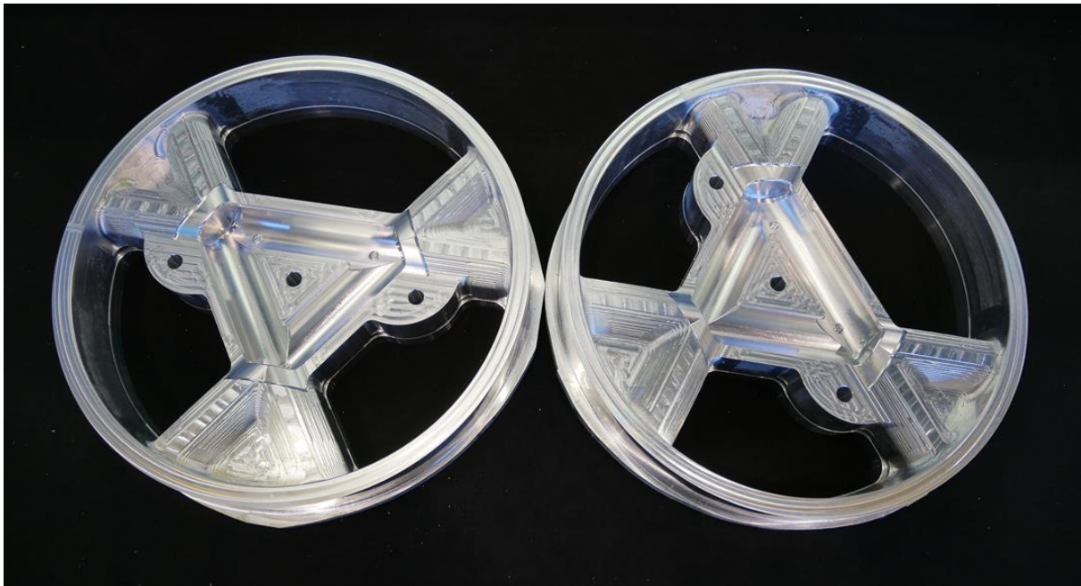
Figure 3.7: Pre-welding stage of the vacuum vessel
