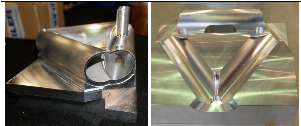
Figure 3.4: Pre-milled moderator (left) & negative form (right)
