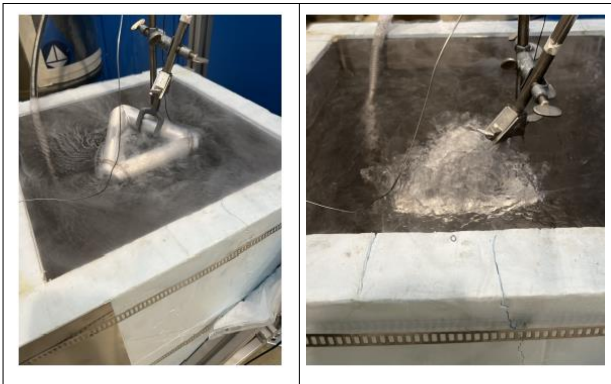
Figure 5.25: Picture of the moderator shortly before it is immersed into liquid nitrogen (left) and in the immersed state (right).
