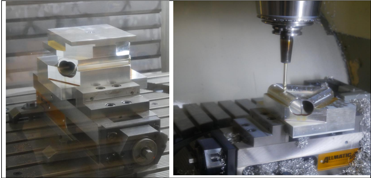
Figure 3.5: Final machining of the hydrogen vessel
