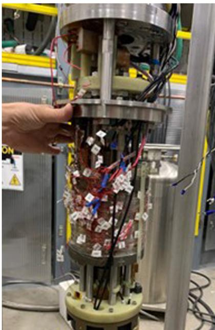
**FIG. 2.** A recent REBCO test coil at the MagLab that includes more advanced structural reinforcement and quench protection than the 32 T user magnet.
