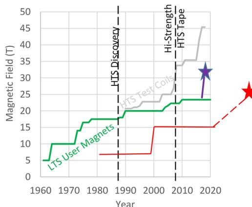
**FIG. 3.** Peak fields available worldwide from a variety of superconducting magnets. LTS solenoids (green), HTS solenoid test coils (gray), HTS user solenoids (purple), and split user magnets (red). By using the HTS technology similar to that used in the MagLab's 32 T solenoid, a split magnet for neutron scattering at a field >20 T should be feasible.
