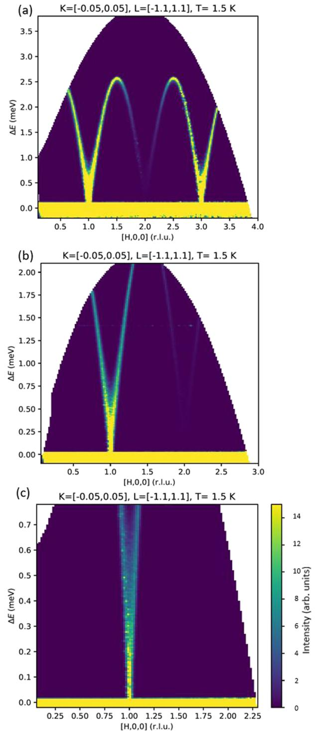
**FIG. 7.** Spin wave simulations for  $K_2V_3O_8$  at incident energies 4.0 meV (a), 2.38 meV (b), and 1.45 meV (c) as in the rep-rate multiplication configuration indicated in Fig. 5. For a 1 g sample, 4 h is needed for a complete measurement (8 settings,  $2^\circ$  steps, and 2 magnet orientations, integrated over all  $L$ ) of the 2D magnetic excitation spectrum. Simulated results using McStas and McVine.
