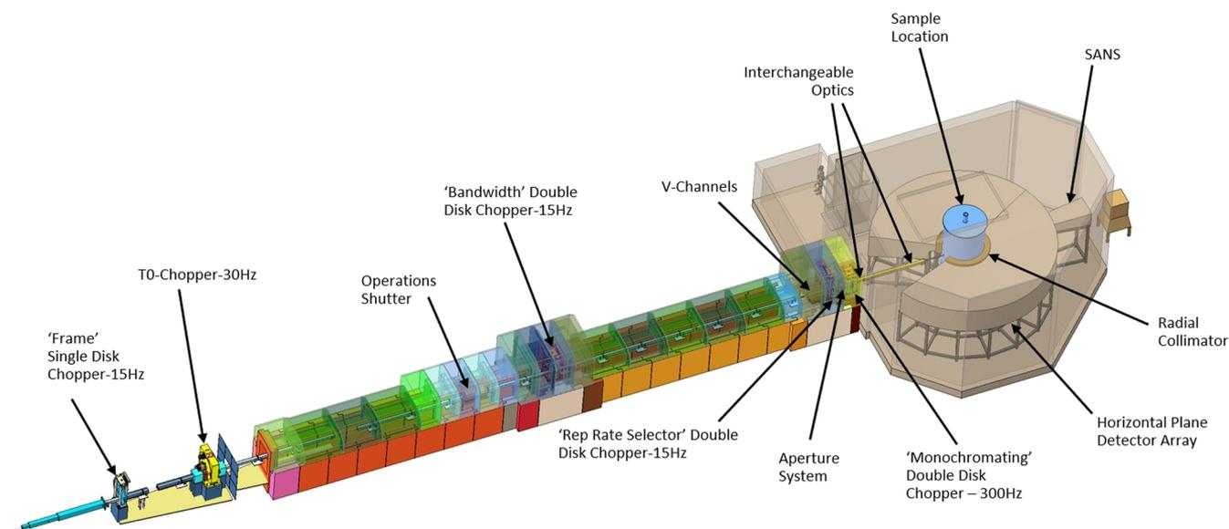
FIG. 6. Overview of entire spectrometer. Chopper frequencies are noted in the labels.
