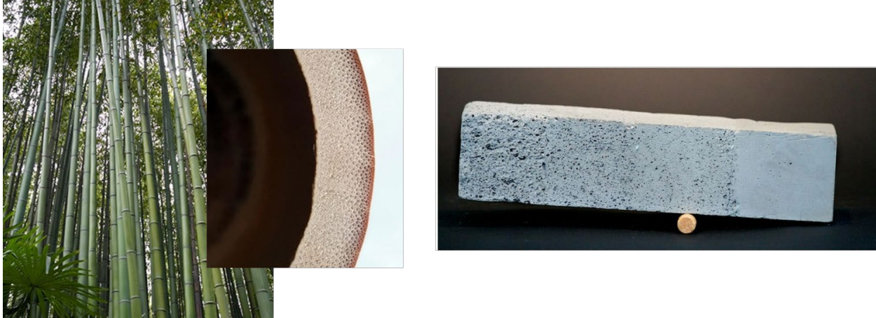
Figure.9;8; Bioinspired functionally graded material with porosity gradient across the depth of the print. The built system allows for strong weather resistance on one surface while integrating both structural efficiency in bending (highest density at outermost fiber of structure) and insulating characteristics into an otherwise highly thermally conductive material.
