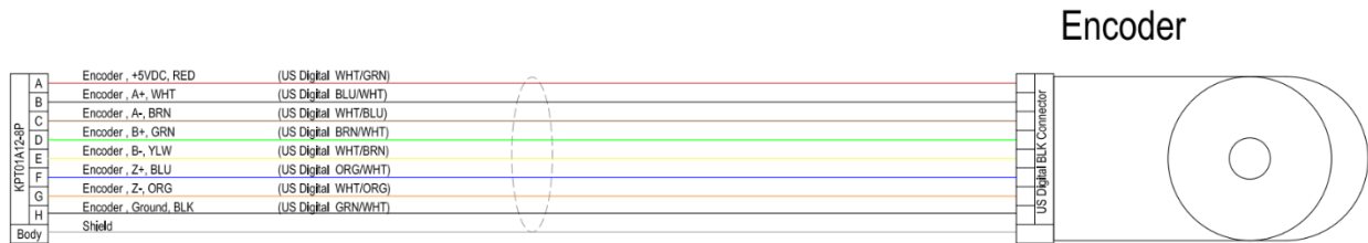
Figure 11: Standard SNS incremental encoder wiring and connector
