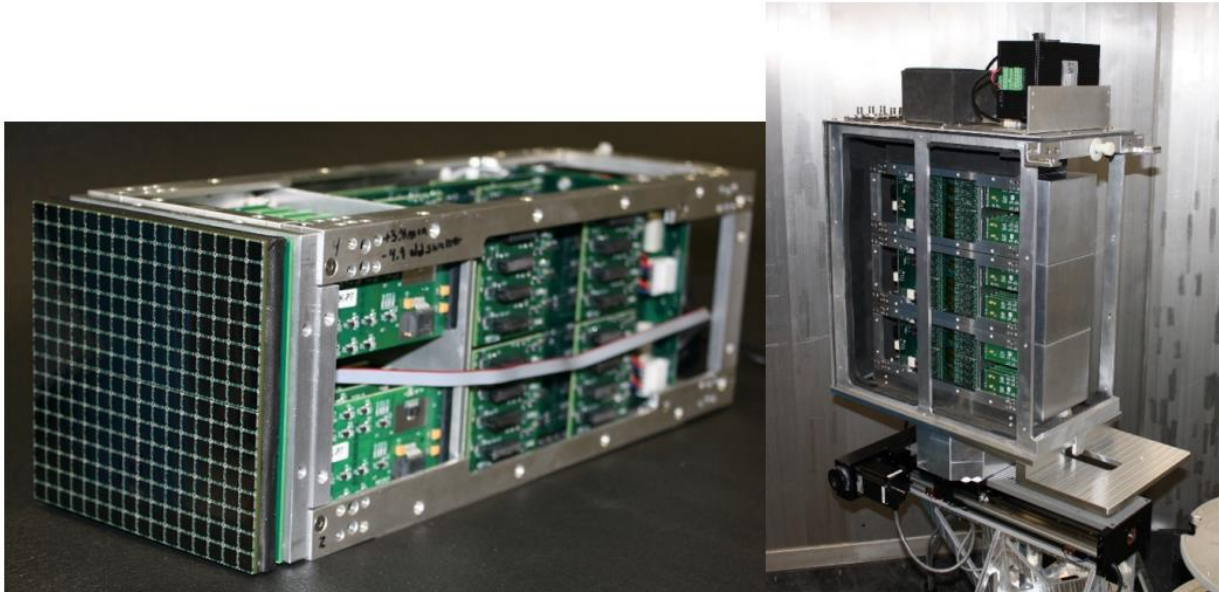
Figure 5: SiPM Anger camera and an array of 3 cameras installed at HFIR [4].
