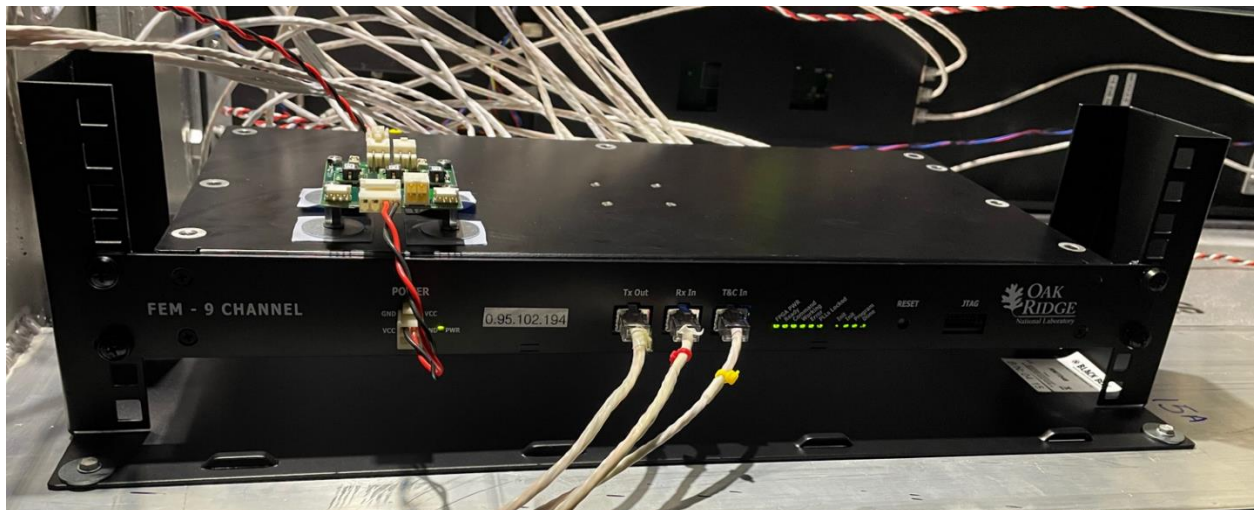
Figure 3: FEM data aggregation module (the front shows the remote communication interface for a data acquisition system and the rear cables are originating from several ROC modules in 8-pack detectors)
